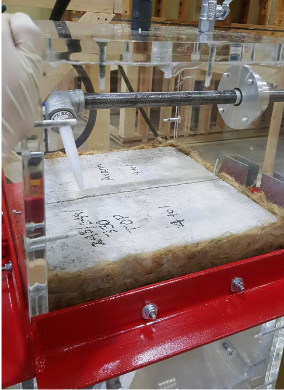
Figure 4. Injection rod and grout nozzle installed
