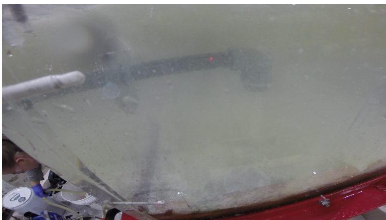
Figure 21- Post-testing: cured grout floats but water is fairly clear
