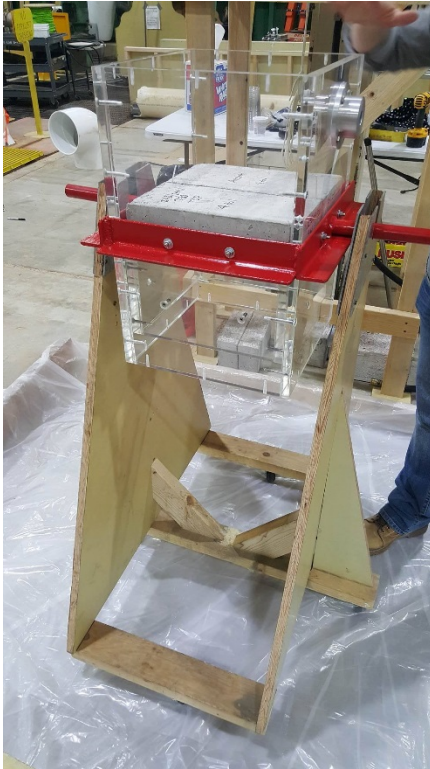
Figure 2. Concrete specimen and chamber in chamber support frame
