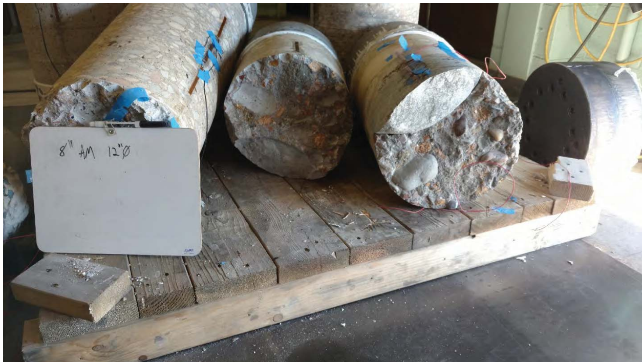
Figure I-2: 12-inch diameter core
