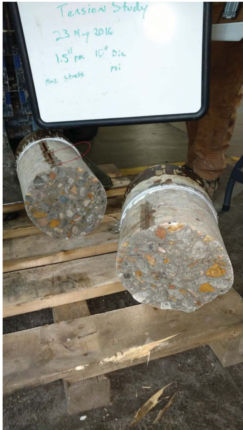
Figure H-9: 10-inch diameter core
