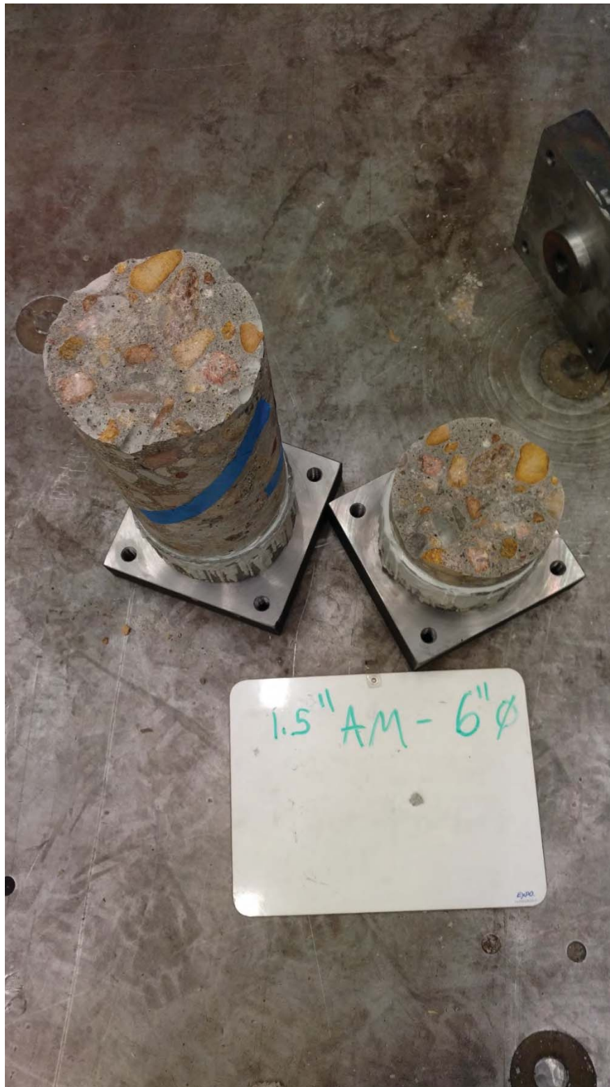
Figure I-11: 6-inch diameter core
