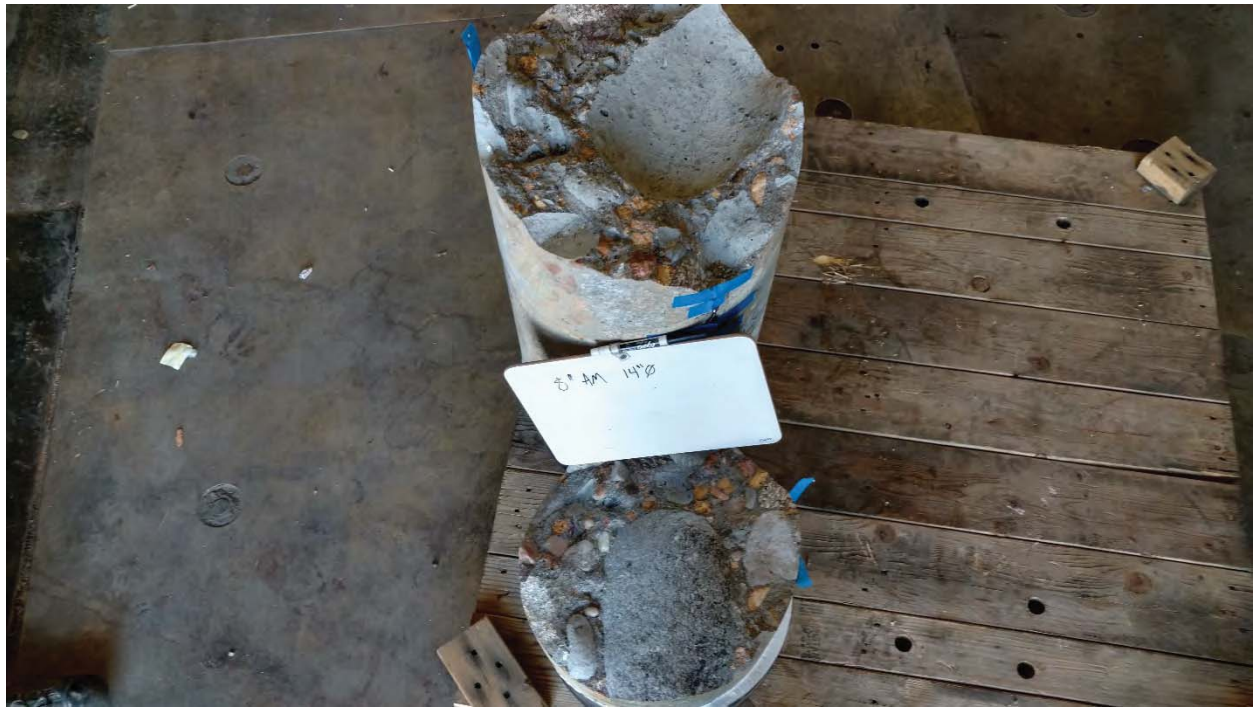
Figure I-1: 14-inch diameter core
