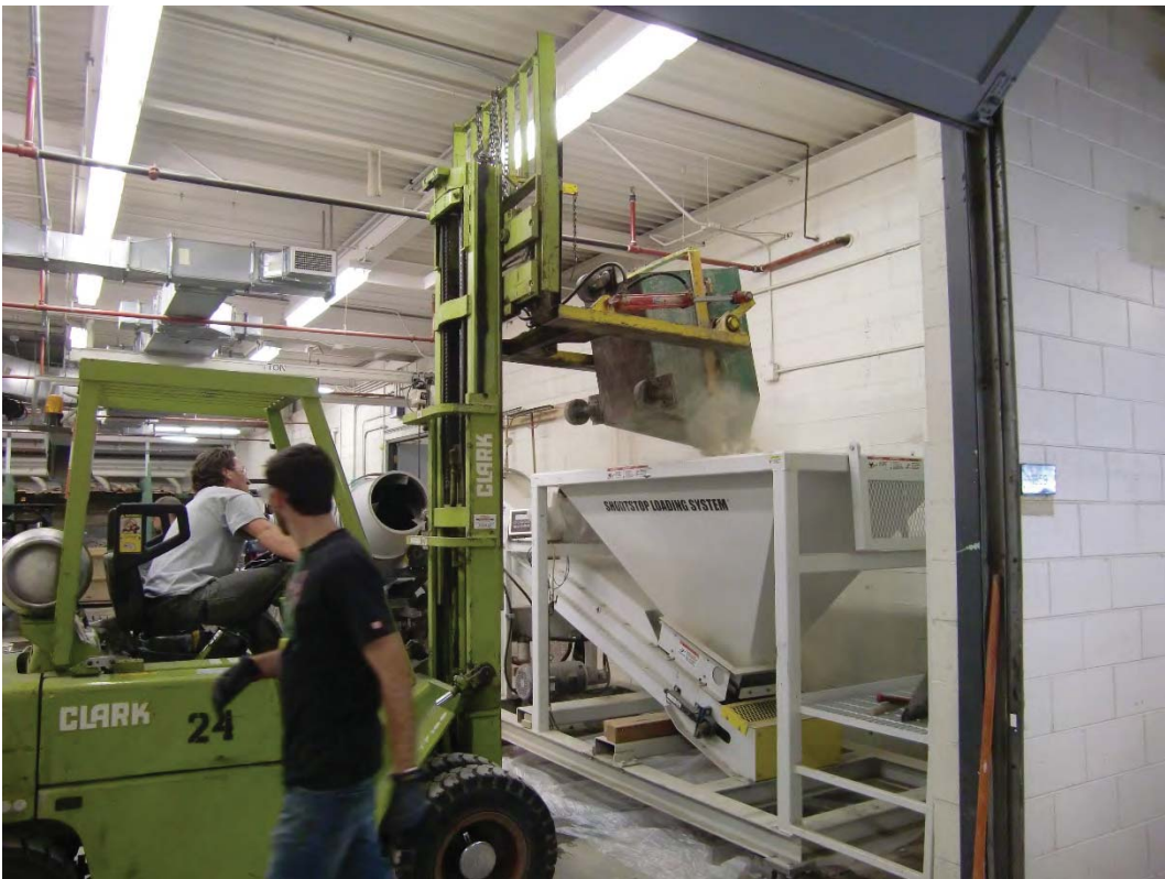
Figure D-2: Placing aggregates into concrete mixer loading hopper
