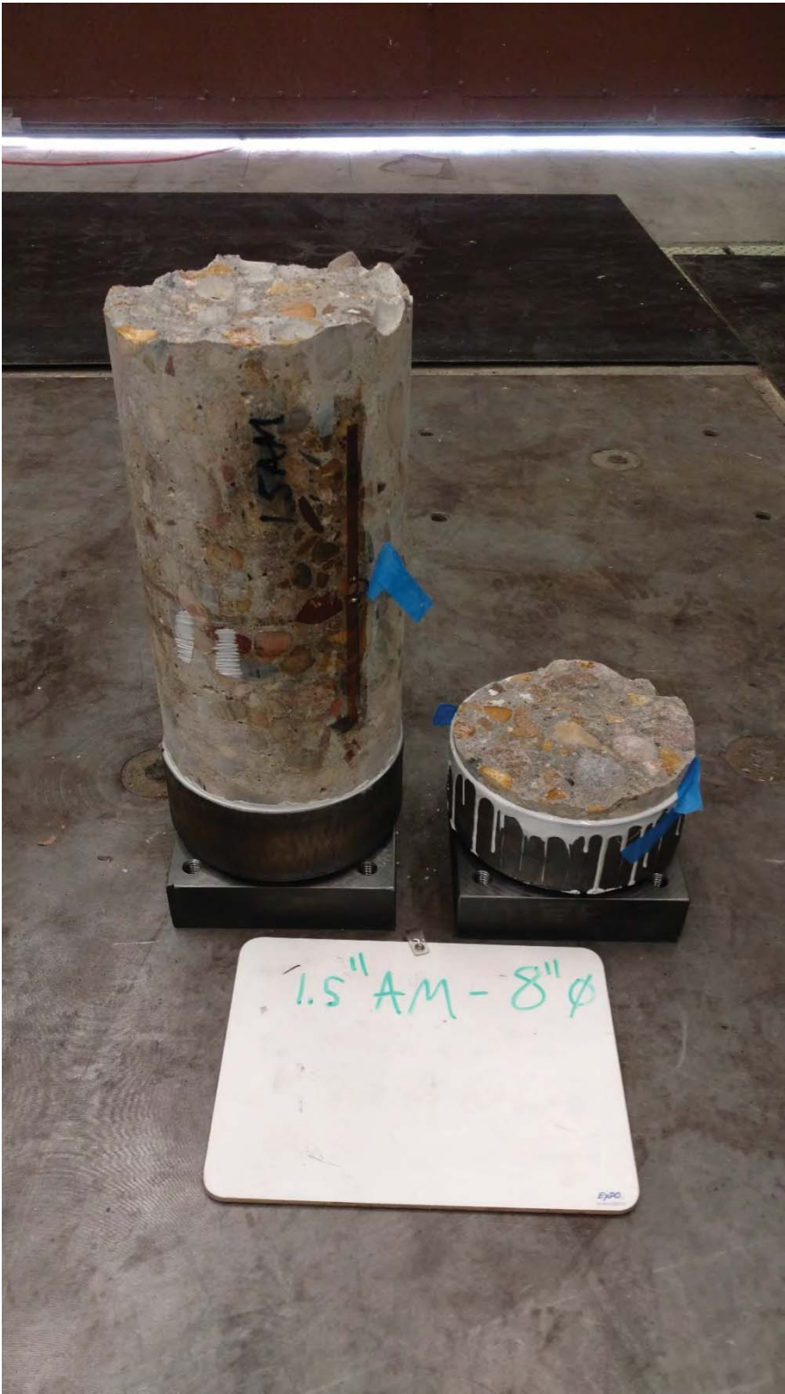
Figure I-10: 8-inch diameter core
