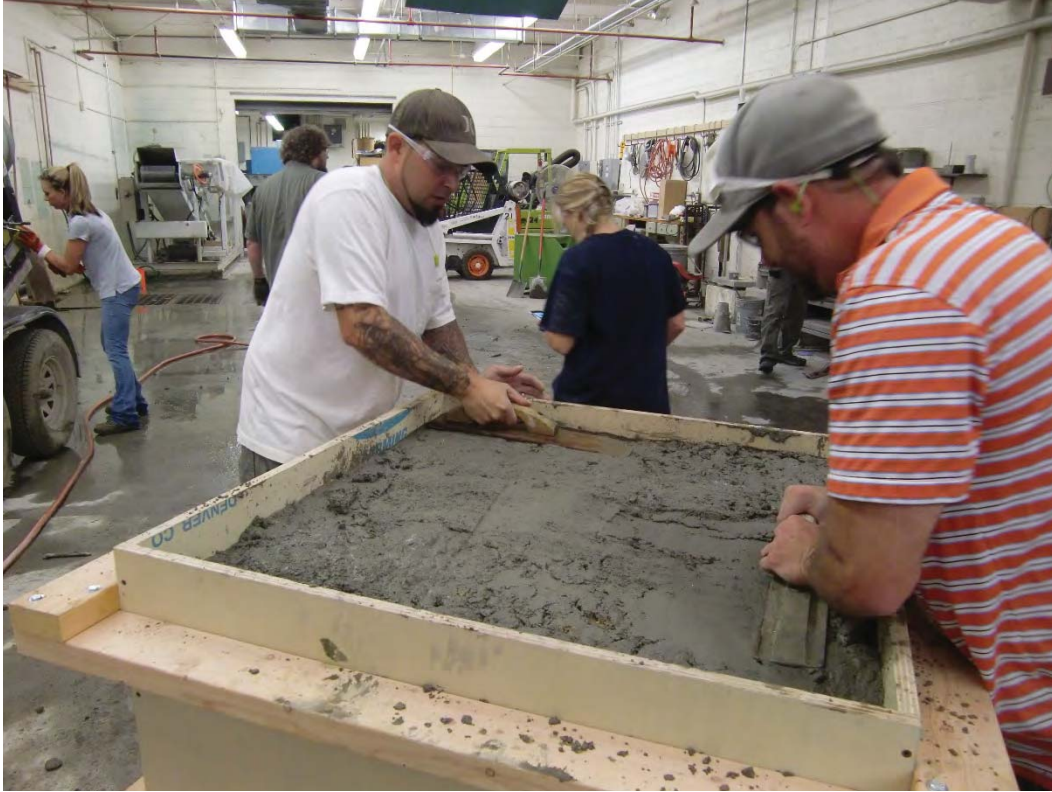
Figure D-11: Finishing 8-inch NMSA concrete block
