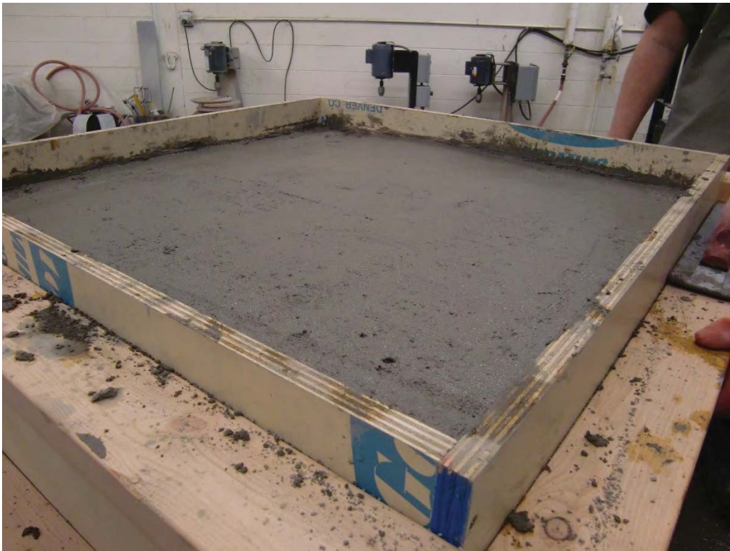
Figure D-12: Completed 8-NMSA concrete block
