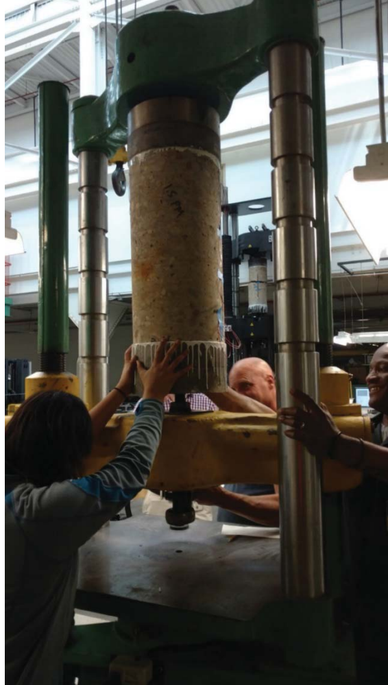
Figure 6 – Static direct tension test setup (12-inch diameter core from 1½-inch NMSA concrete mix shown)
