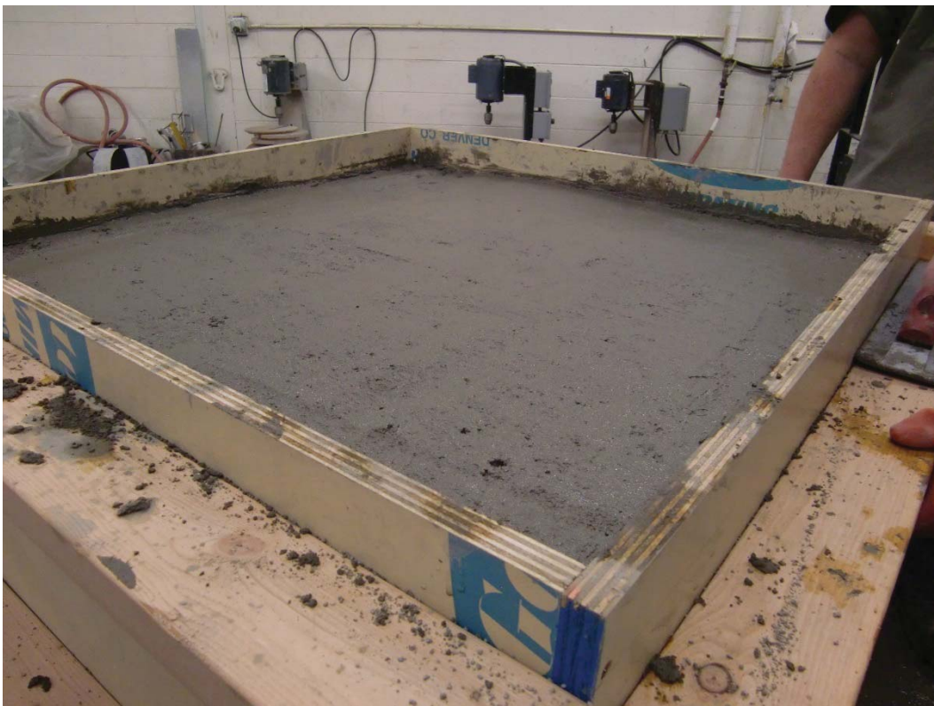
Figure 2 – Completed 8-inch NMSA concrete block
