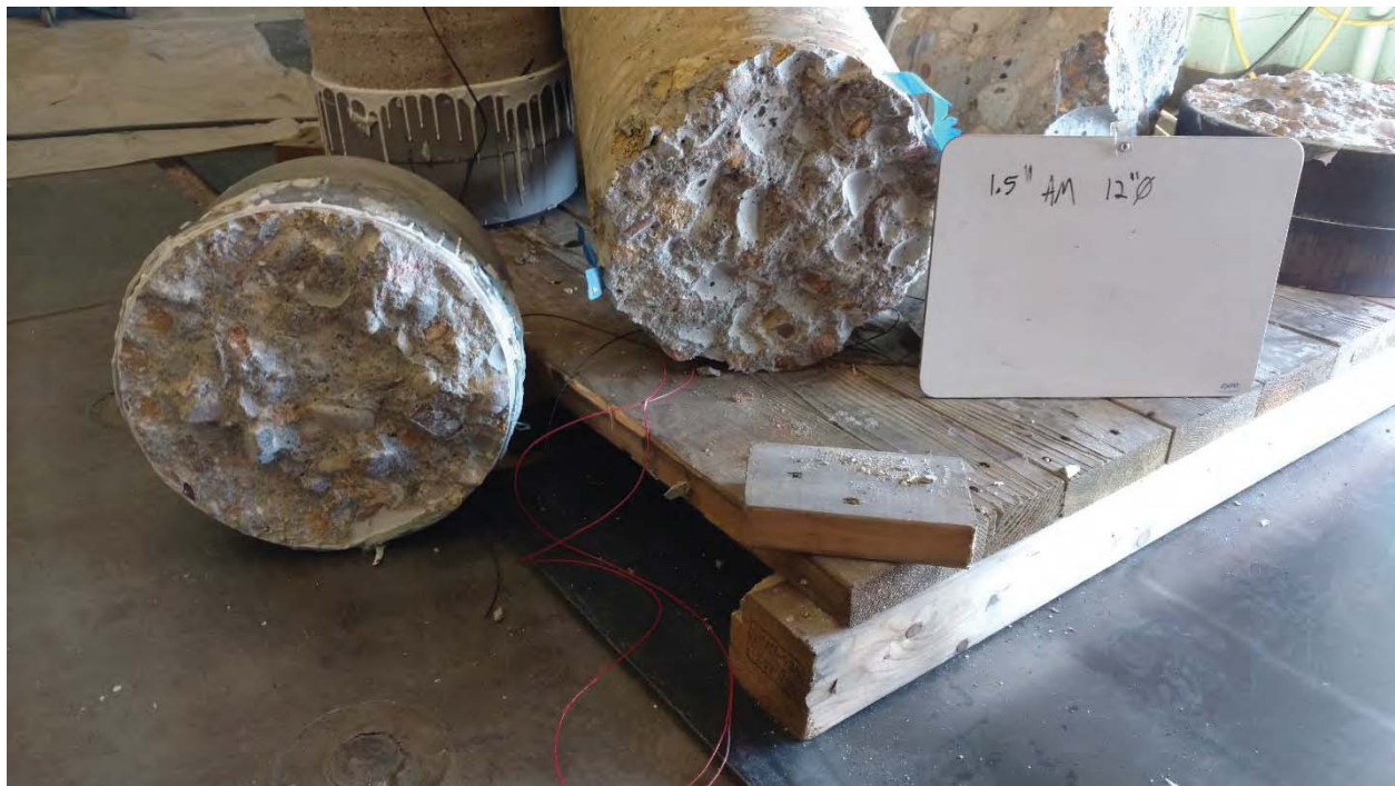
Figure I-8: 12-inch diameter core
