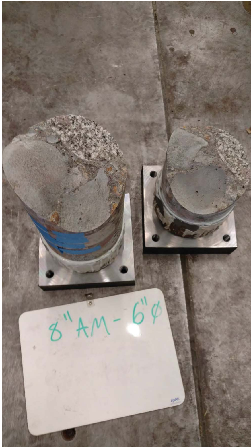
Figure I-5: 6-inch diameter core
