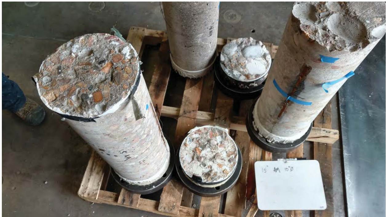
Figure I-9: 10-inch diameter core
