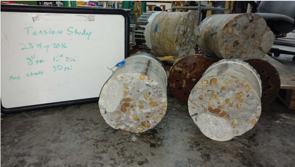
Figure H-3: 10-inch diameter core
