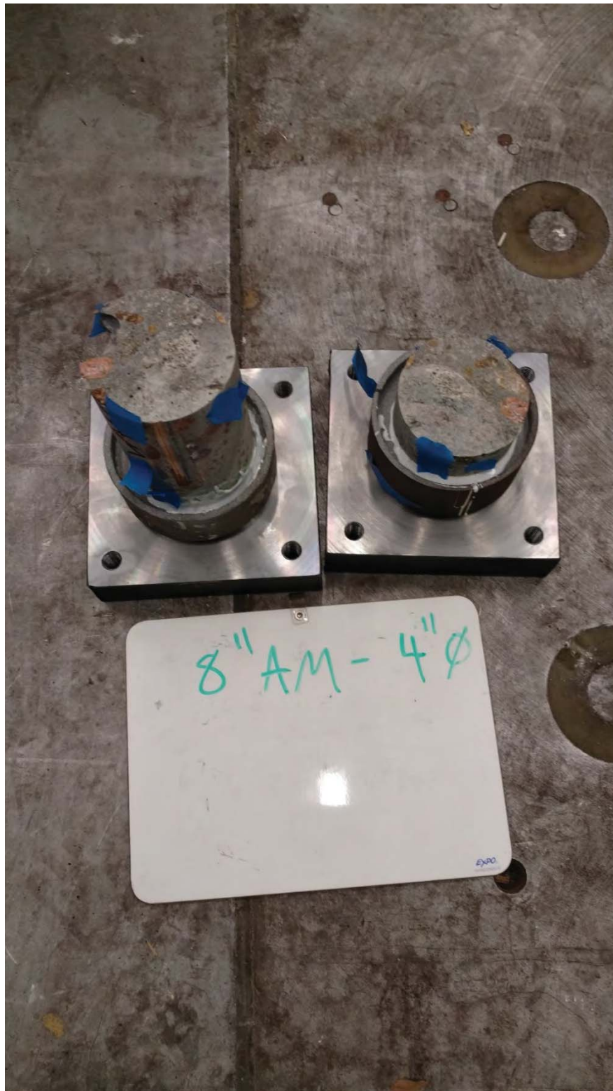
Figure I-6: 4-inch diameter core
