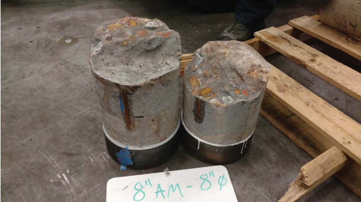
Figure I-4: 8-inch diameter core
