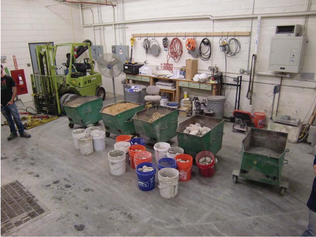
Figure D-1: Batched aggregates for 8-inch NMSA blocks
