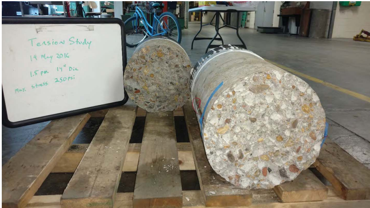
Figure H-7: 14-inch diameter core
