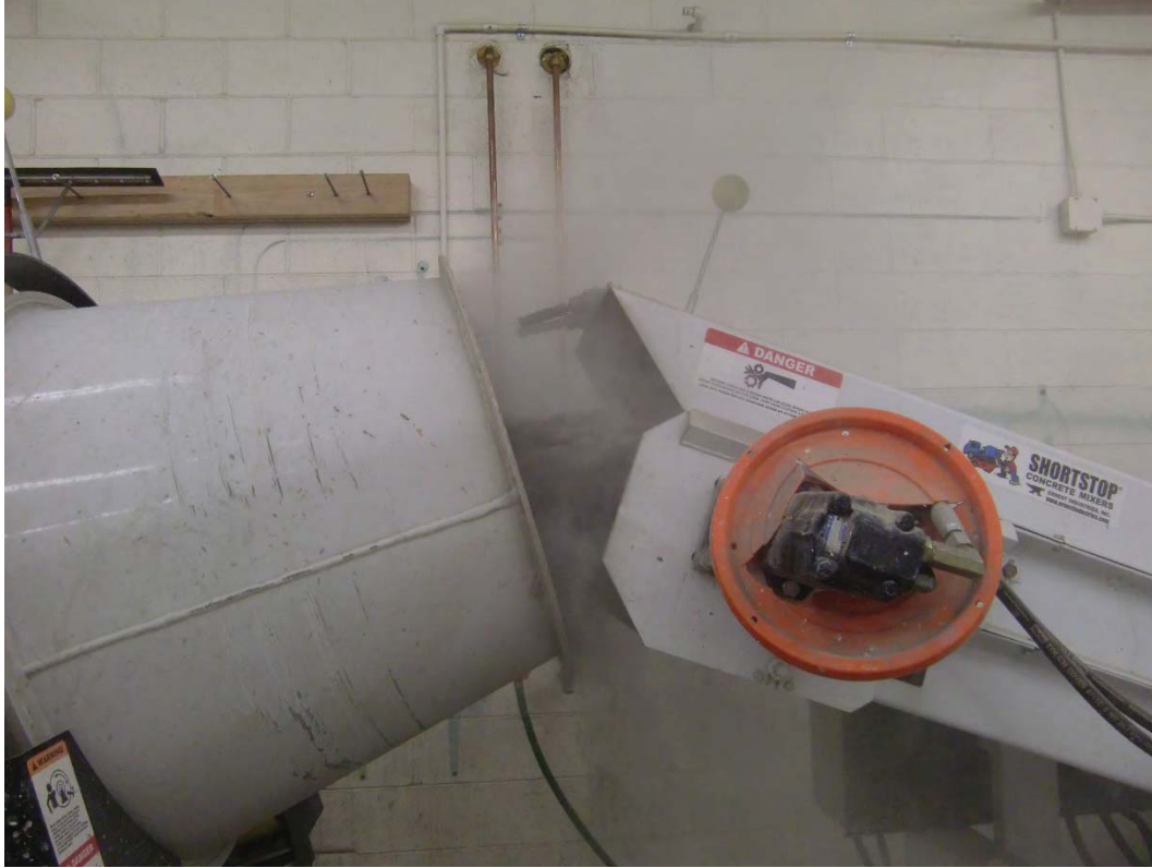
Figure D-3: Hopper loading 1-cubic yard concrete mixer
