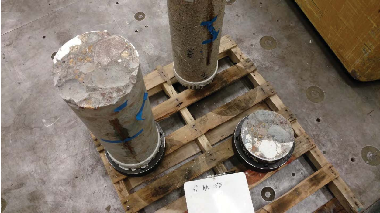
Figure I-3: 10-inch diameter core
