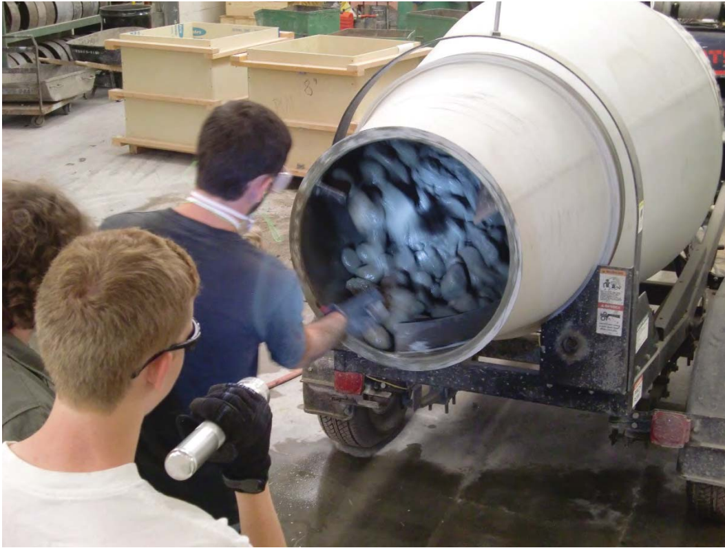
Figure D-5: 8-inch NMSA concrete mixing (note that 4- to 8-inch
