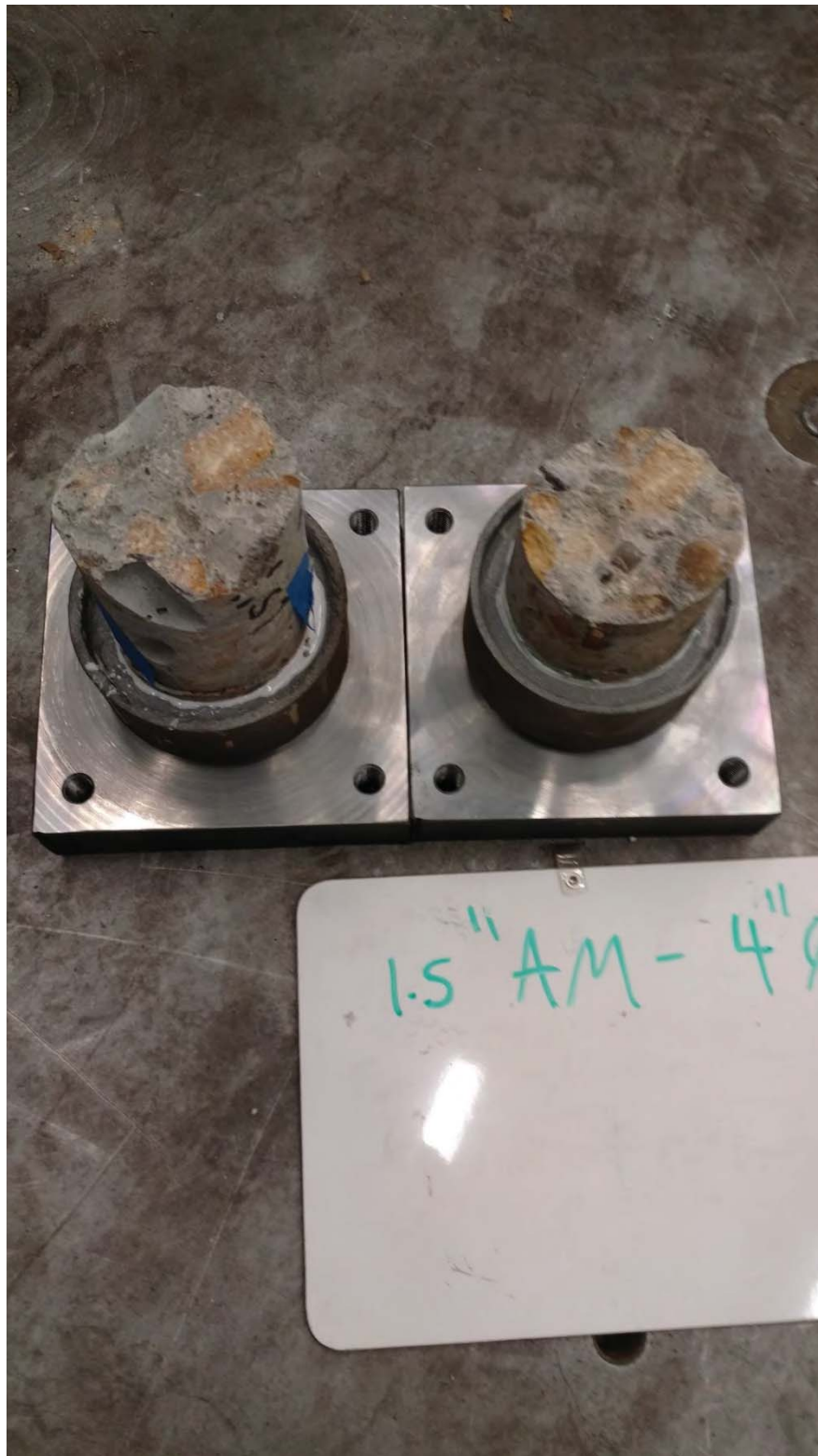
Figure I-12: 4-inch diameter core
