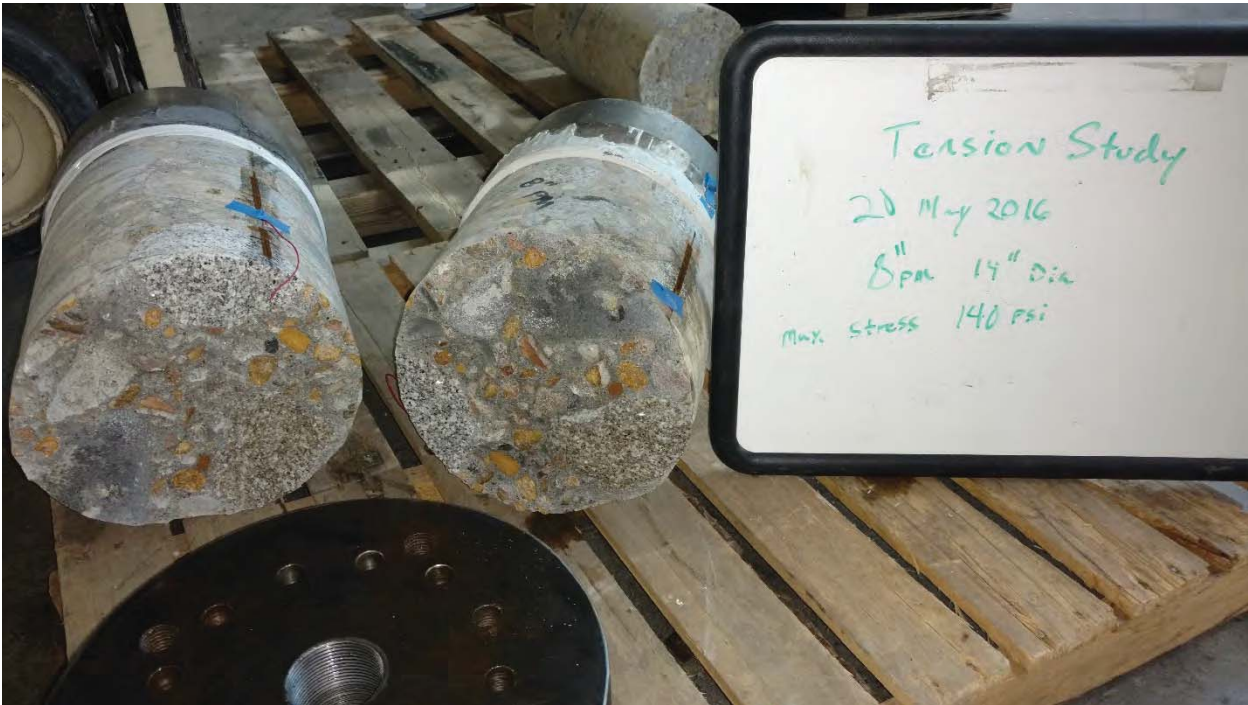
Figure H-2: 12-inch diameter core
