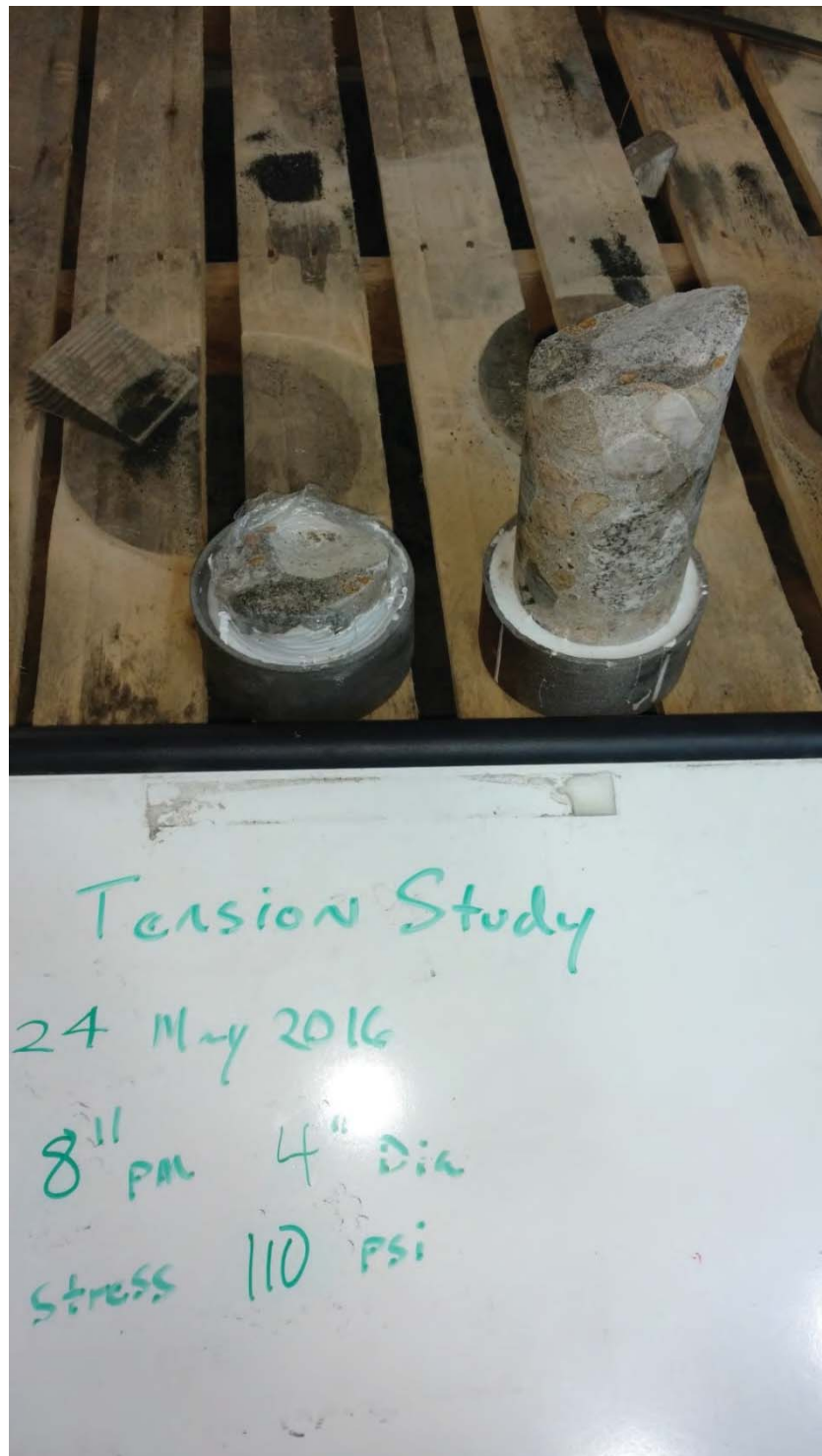
Figure H-6: 4-inch diameter core
