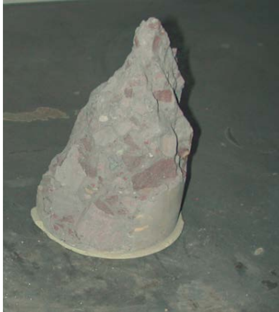
Figure 6.2.—Geometry typical of a failed cylinder from UXC Unconfined Test (Photo by Harris; courtesy of Materials Engineering and Research Laboratory)
