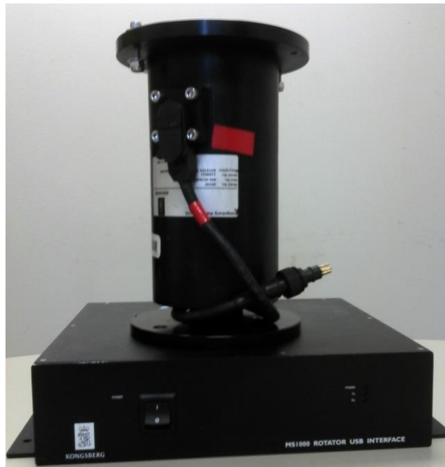
Figure 6.—Kongsberg Mesotech Ltd single-axis mechanical rotator with communication/power interface unit.
