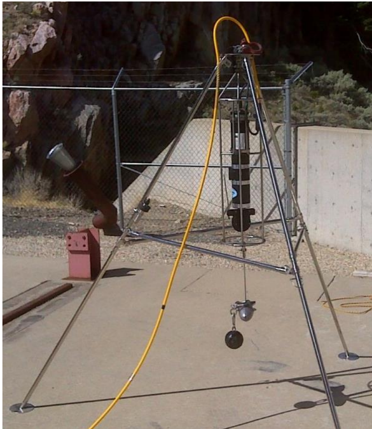
Figure 10.—Gimbal-mounted scanning sonar on a tripod. This tripod system will produce a vertical orientation on an uneven or sloped surface.
