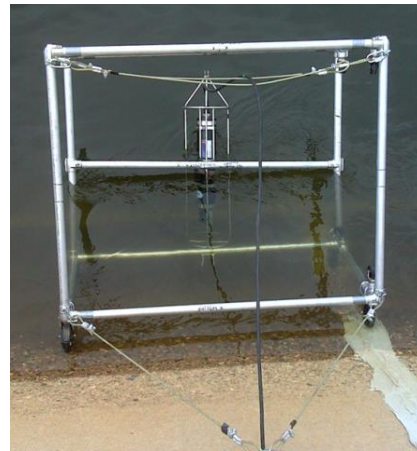
Figure 13.—Custom wheeled cart that is used to lower the sonar down a sloped concrete surface to image the canal lining.
