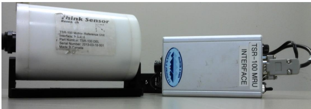
Figure 7.—Think Sensor Research TSR-100 MRU (left) and a communications/power interface.
