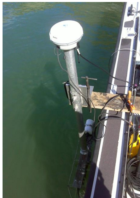
Figure 15.—Photograph of a pole-mounted sonar with an external MRU (white cylinder) that was used during a bathymetric survey.
