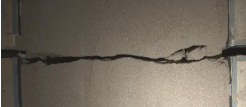
Figure 13.—Overhead view of Test 6: 3 feet of sand compacted to 92.9%.
