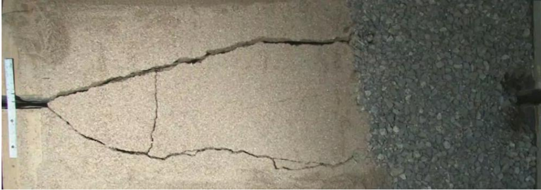
Figure 19.—Overhead view of Test 11: 3 feet of sand compacted to 89.3% and 2 feet of compacted gravel.
