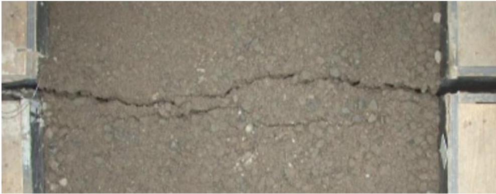
Figure 15.—Overhead view of Test 8: 3 feet of broadly graded material compacted to 103.4%.
