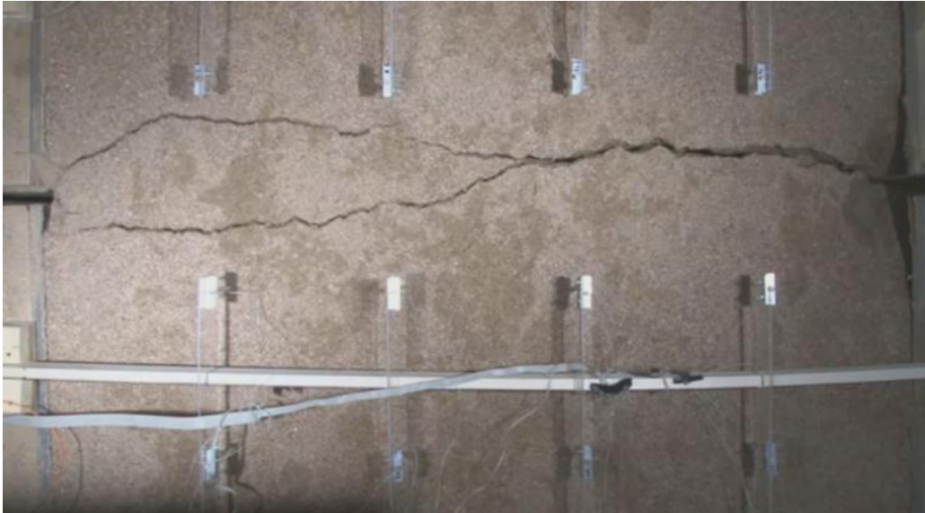
Figure 20.—Overhead view of Test 12: 5 feet of sand compacted to 92.9%.
