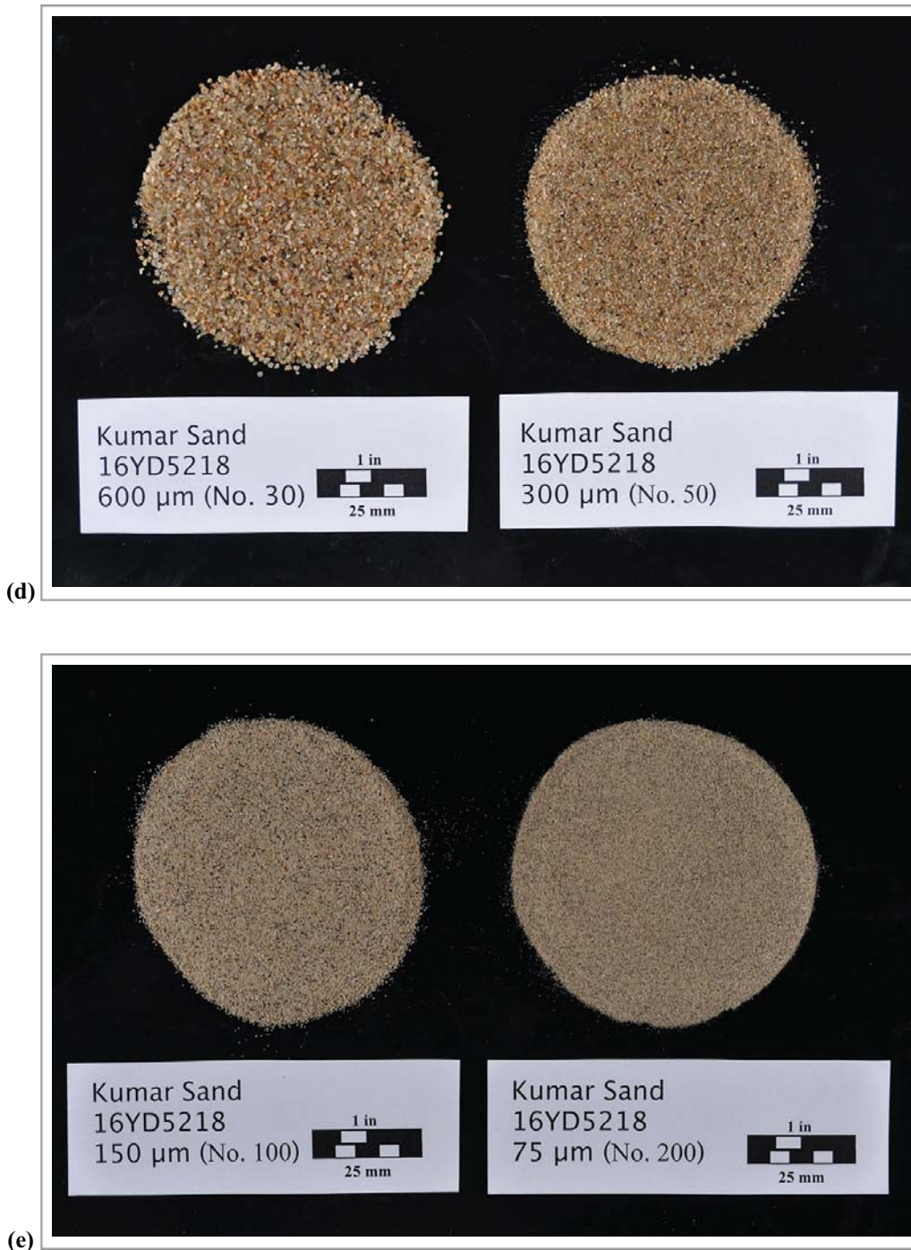
Figure 2 (cont'd). Photographs of concrete sand showing fractions retained on the (d) 600 \mu\text{m} (#30) sieve and 300 \mu\text{m} (#50) sieve and the (e) 150 \mu\text{m} (#100) and 75 \mu\text{m} (#200) sieves.
