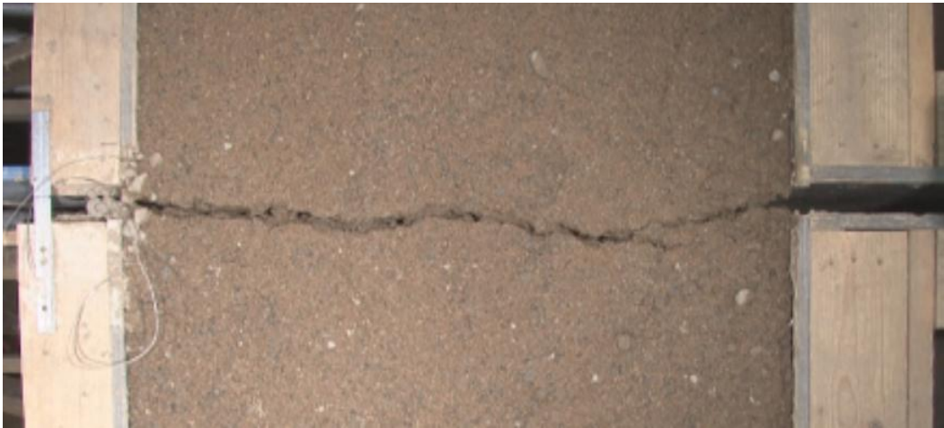
Figure 17.—Overhead view of Test 9: 3 feet of broadly graded material compacted to 92.5%. (Note: the materials in tests 7, 8, and 9 are identical. The lighting in each photo affects the appearance of the material.)
