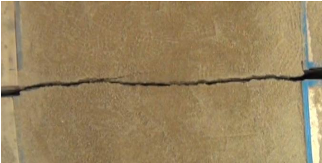
Figure 22.—Overhead view of Test 14: 3 feet of sand compacted to 91.3%.
