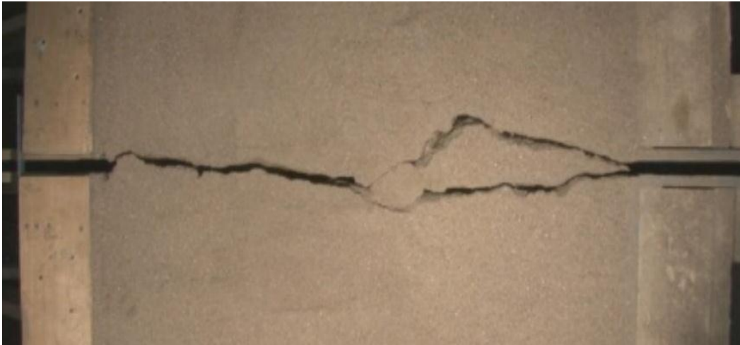
Figure 10.—Overhead view of Test 3: 3 feet of sand compacted to 95.7%.
