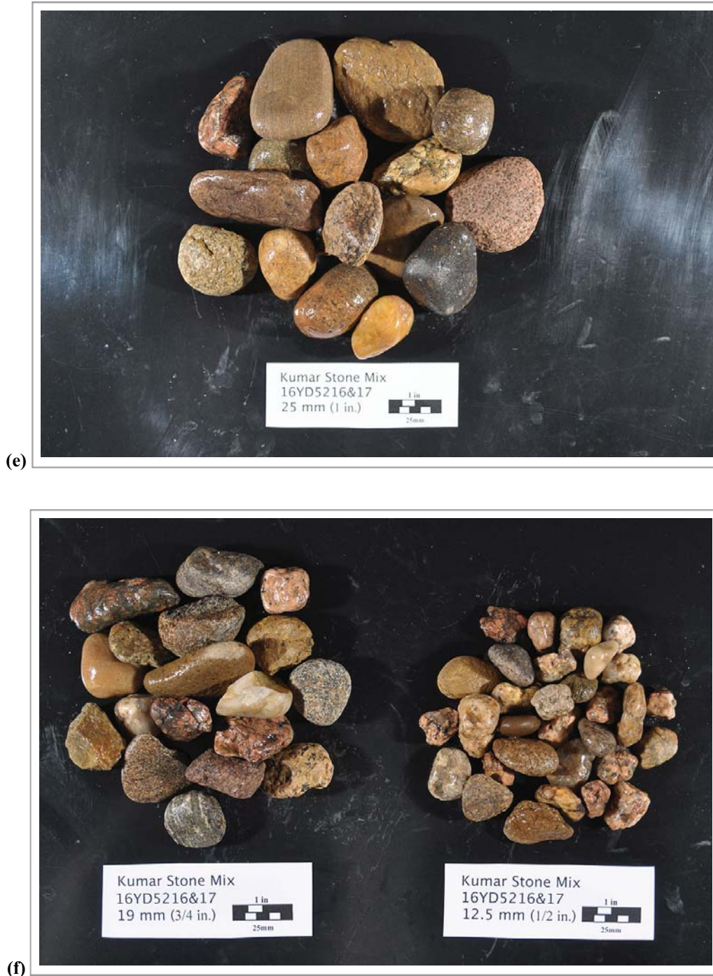
Figure 1 (cont'd). Photographs of #467 stone showing fractions retained on the (e) 25 mm (1 in.) sieve and the (f) 19 mm (3/4 in.) and 12.5 mm (1/2 in.) sieves.
