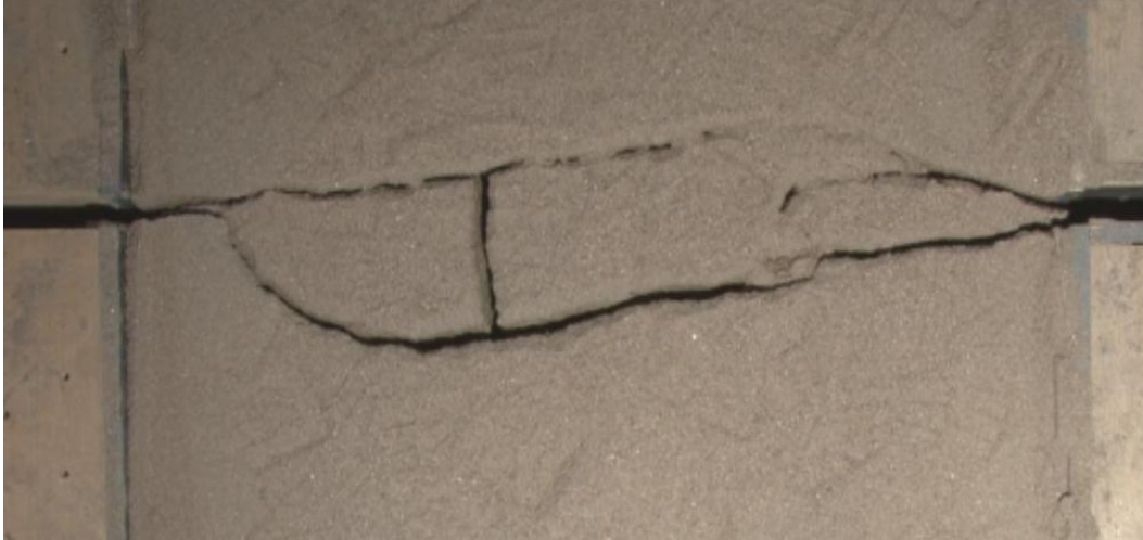
Figure 11.—Overhead view of Test 4: 3 feet of sand compacted to 87.6%.
