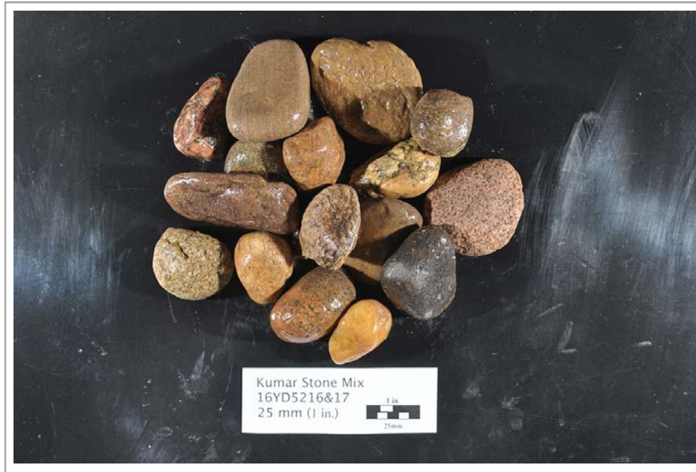
Figure 1 (cont'd). (g) Photograph of #467 stone showing fractions retained on the 9.5 mm (3/8 in.) sieve and the 4.75 mm (#4) sieve.
