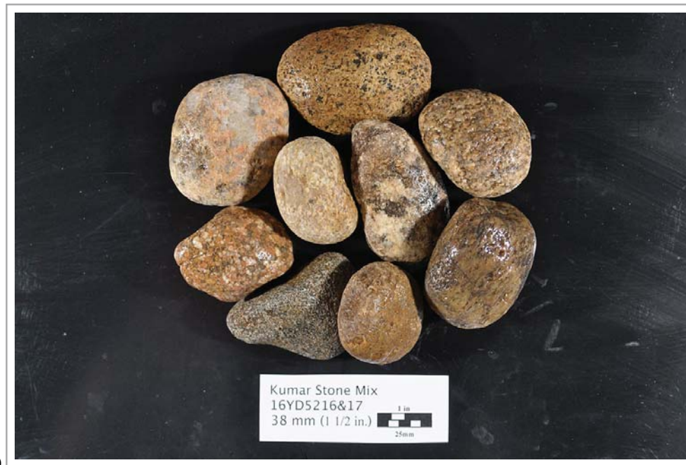
Figure 1 (cont'd). (c) Photograph of #467 stone derived from mixing the #4 stone and the #57/67 stone. (d) Photograph of fraction retained on the 38 mm (1 1/2 in.) sieve.
