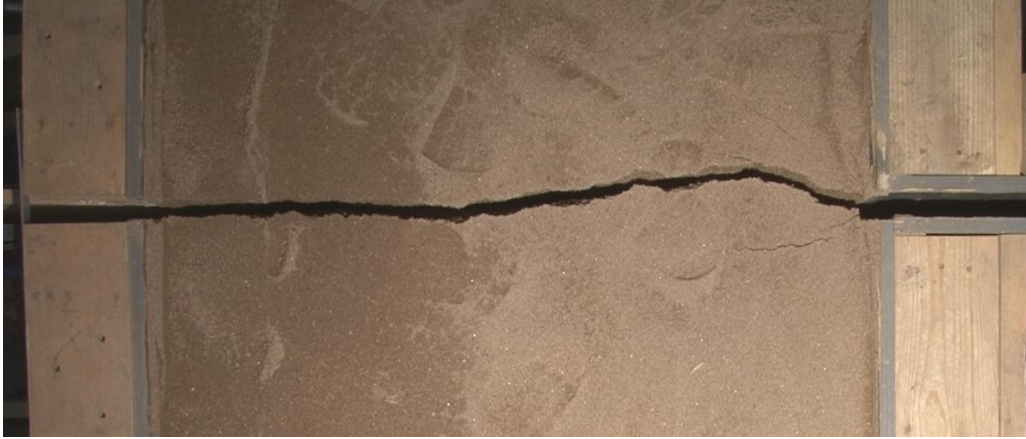
Figure 12.—Overhead view of Test 5: 3 feet of sand compacted to 90.6%.
