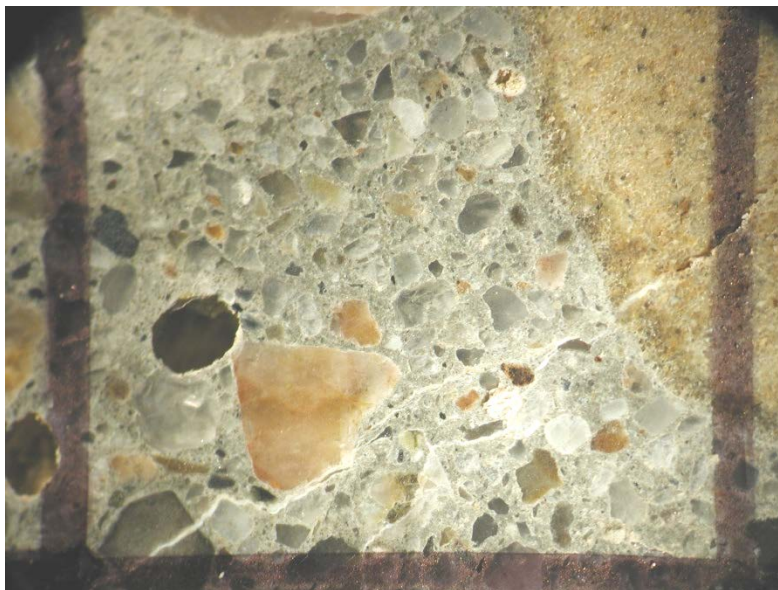
Figure 10. A reactive aggregate particle exhibits an internal crack filled with alkali-silica gel. The filled crack also penetrates paste. The examined square received a count each for coarse aggregate with crack and gel, cement paste with crack and gel, and reaction rim around aggregate (CA+G, CP+G, and R following the defect types of Rivard, 2002). The grid square is about 10 by 10 millimeters in size.
