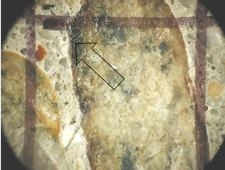
Figure 11 Fresh alkali-silica gel exuded onto the polished surface following sample preparation (arrow). The gel is transparent and the incident light on the irregular surface causes it to sparkle slightly. The grid square is about 10 by 10 millimeters in size.
