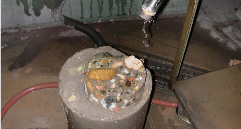
Figure 4. A six-inch diameter concrete specimen sits on a stand during the polishing process. The hose provides limited water to keep the working surface wet and lubricated for polishing.
