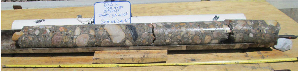
Figure 13 The general condition of concrete core DH-13-2, at depths greater than 5.4 feet for comparison.
