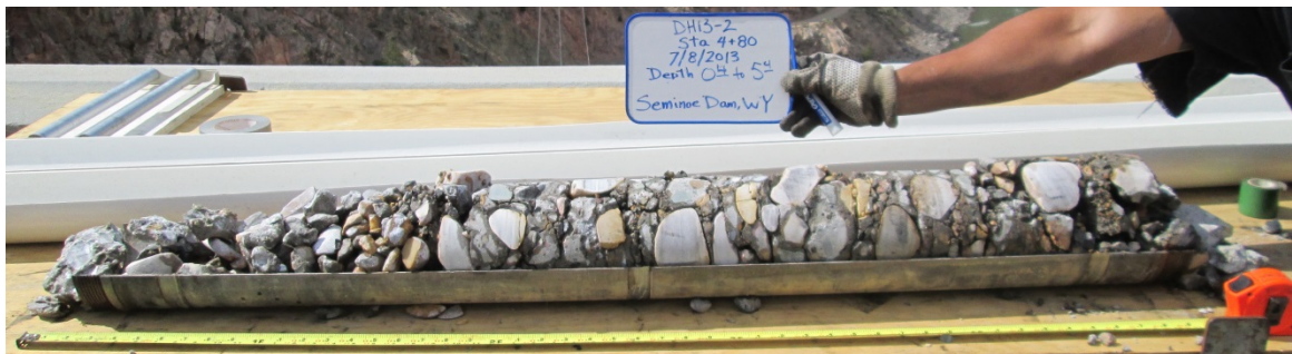
Figure 12 The condition of concrete core DH-13-2, 0.4 to 5.4 feet. The Seminoe Dam core at shallower depths was not available for DRI. The DRI value at the interval 0 to 5.4 feet, if available, would likely be much higher than that observed at greater depths.
