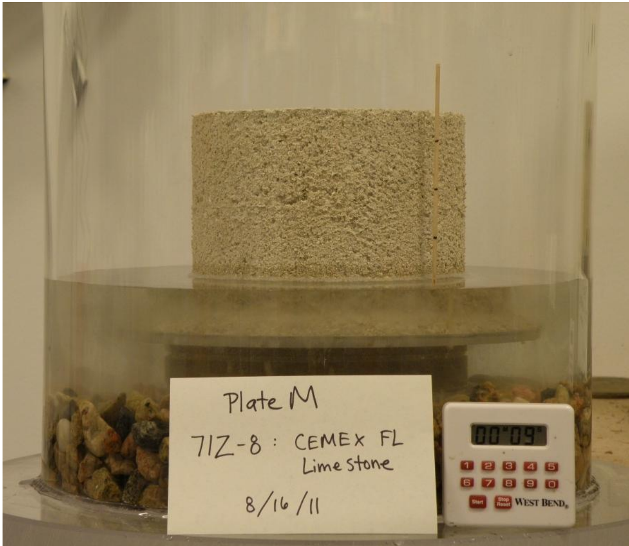
Figure A-61.—Florida Cemex specimen at beginning of Sand Castle Test.
