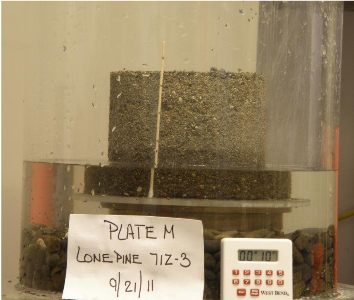
Figure A-39.—Sample shown at start of Sand Castle Test.
