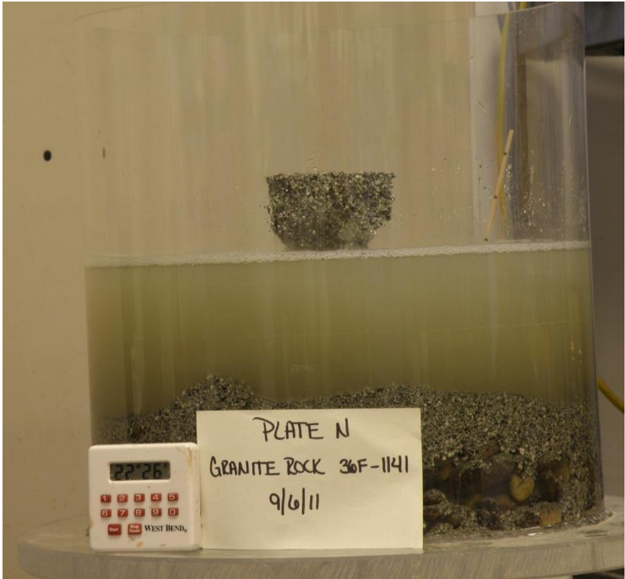
Figure A-25.—A Granite Rock Sand Castle specimen immediately before failure.
