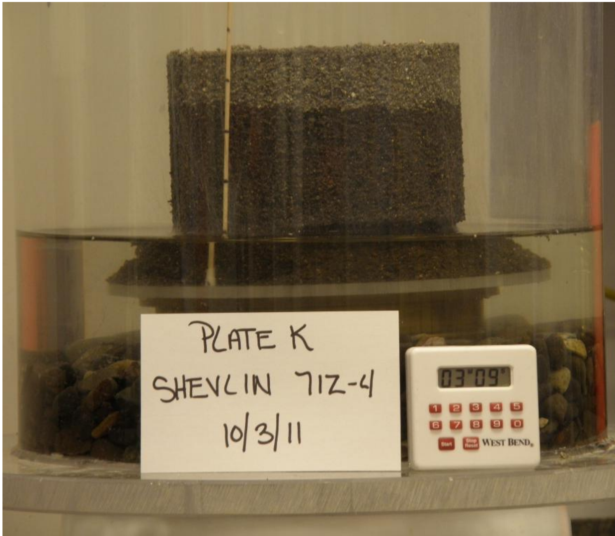
Figure A-44.—Specimen has almost fully absorbed water.
