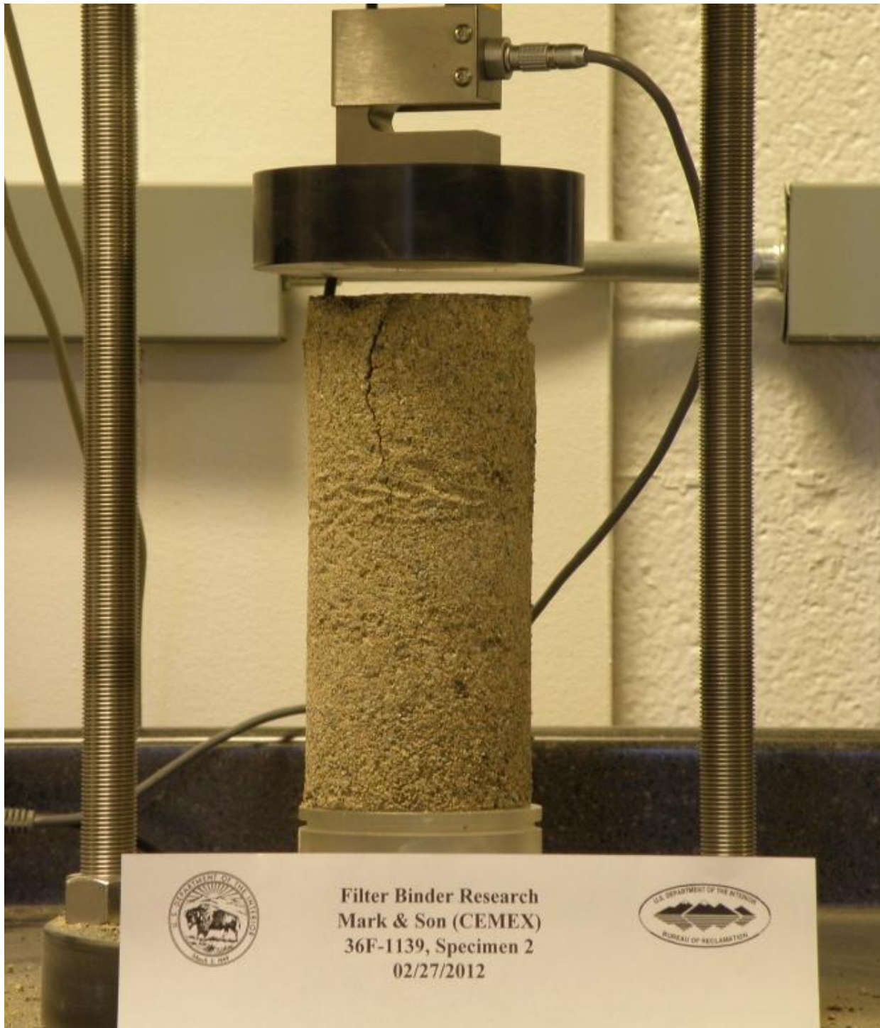
Figure A-18.—Speciment at failure.
