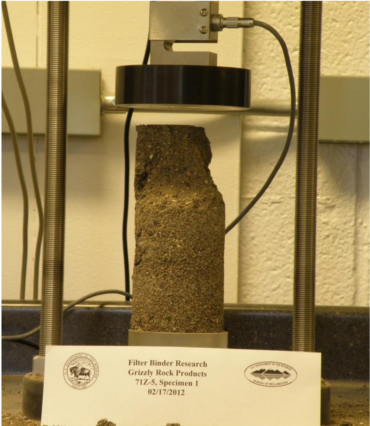
Figure A-52.—Specimen after failure.
