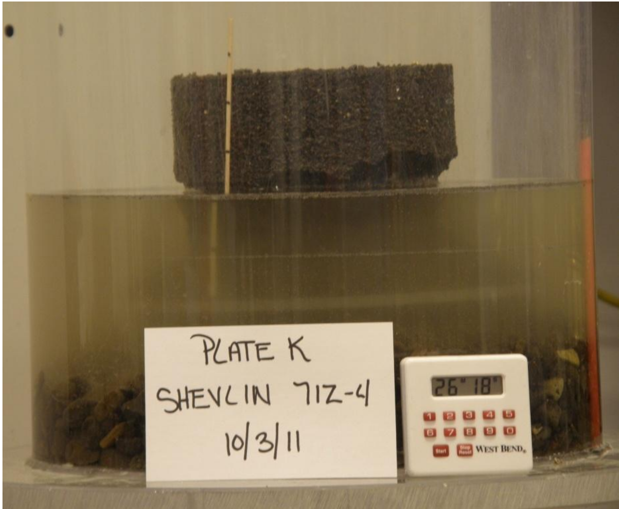
Figure A-45.—Specimen at 50% disintegration after water raised to 2 inches.
