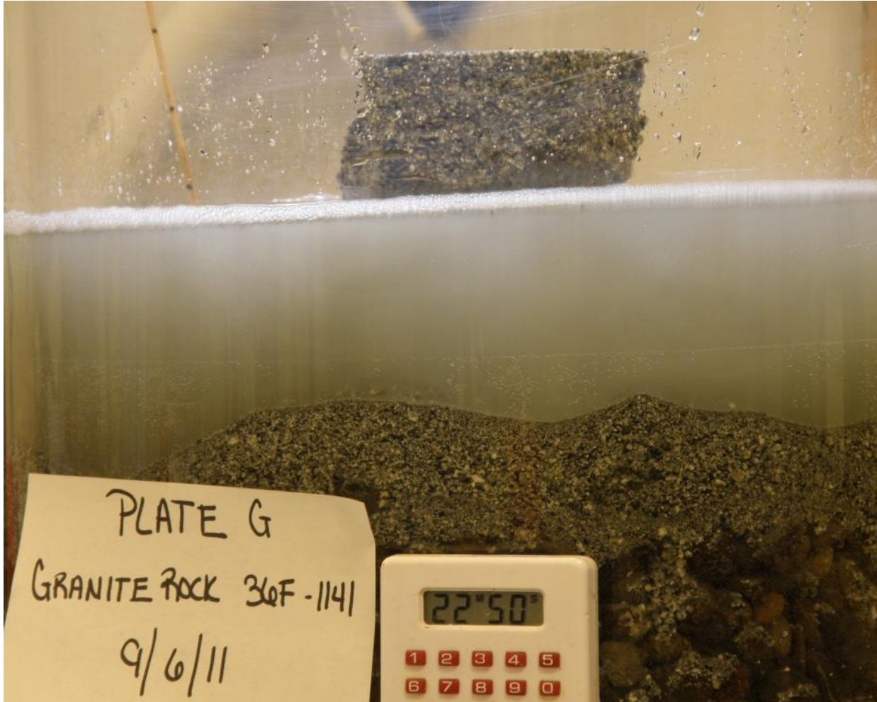
Figure A-24.—Granite Rock Sand Castle Test specimen – a typical representation of specimen immediately before failure.
