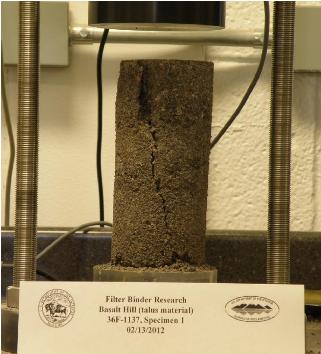
Figure A-9.—Sample showing failure after UCS Test.
