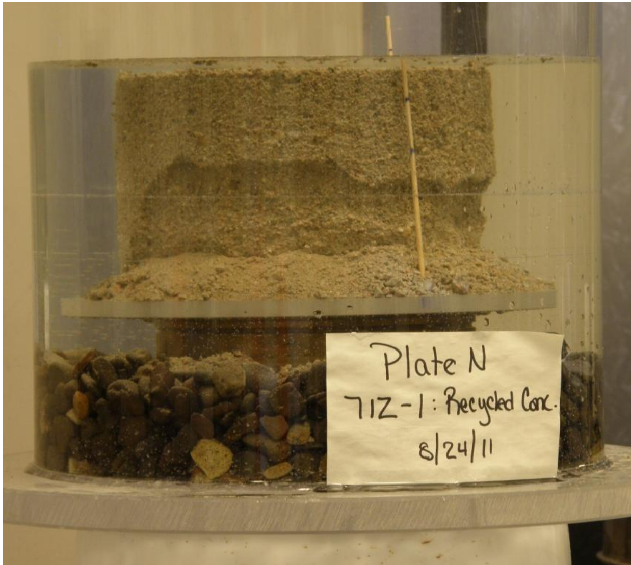
Figure A-31.—Specimen shown completely submerged for over 24 hours. Specimen did not fail during Sand Castle Test.
