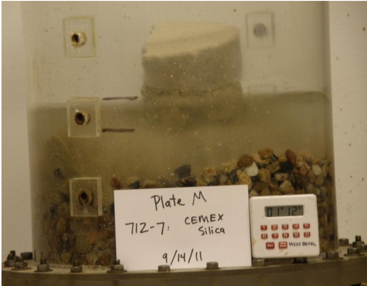
Figure A-58.—Another Cemex “topple” failure.
