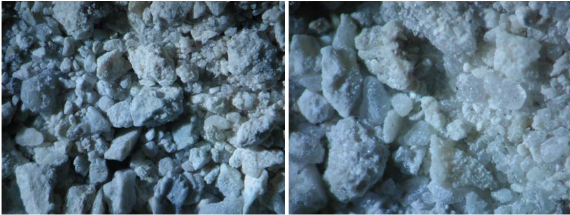
Figure 27. CEMEX Limestone Sand (FL), 71Z-8. The images show the irregular surfaces of as-received specimen fragments at two different magnifications. The particles appear subangular and subrounded in shape. The field on the left image is about 16 mm width and the field on the right is 6 mm width and the corresponding magnification are about 6X and 17X, respectively.
