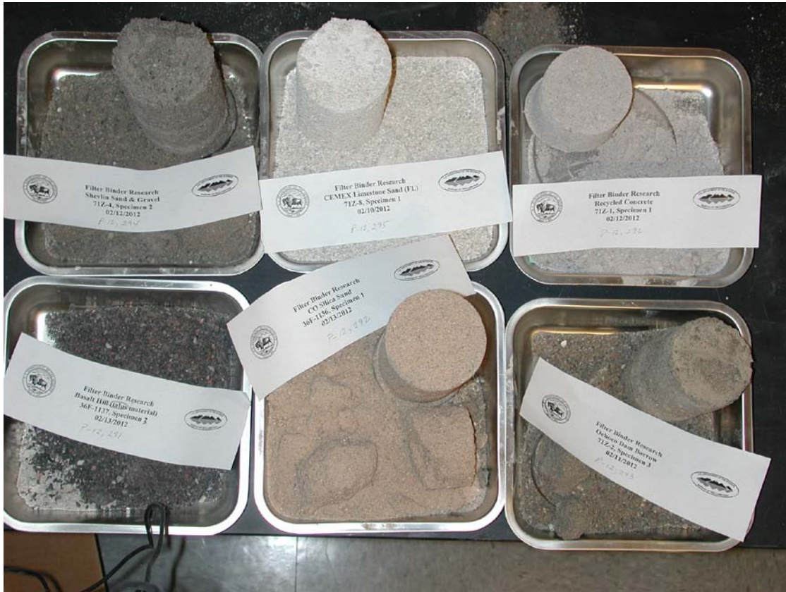
Figure 1. The image shows the submitted filter binder research cylinders after removing material for thin section preparation. Note: Some of the samples completely disaggregated and some are essentially intact after handling.
