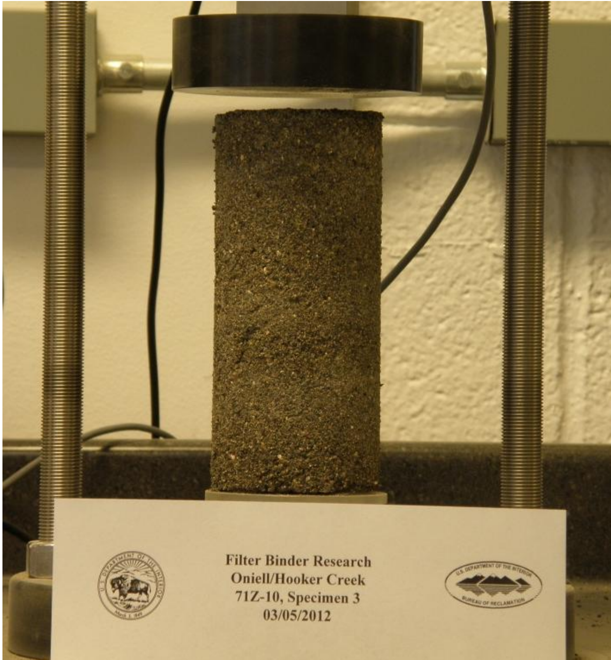
Figure A-75.—Oniell specimen at failure.
