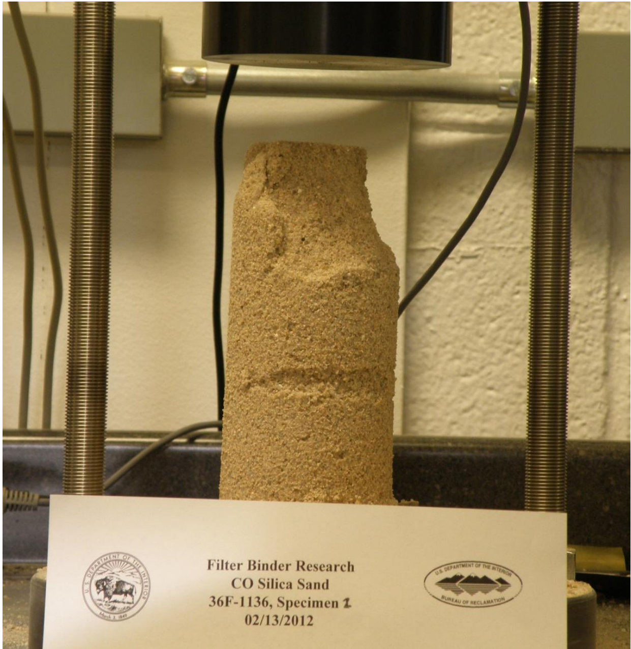
Figure A-4.—Sample showing failure plain after UCS Test.
