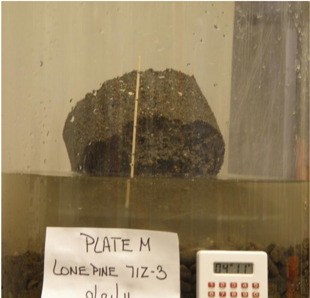
Figure A-41.—Typical “topple” failure.
