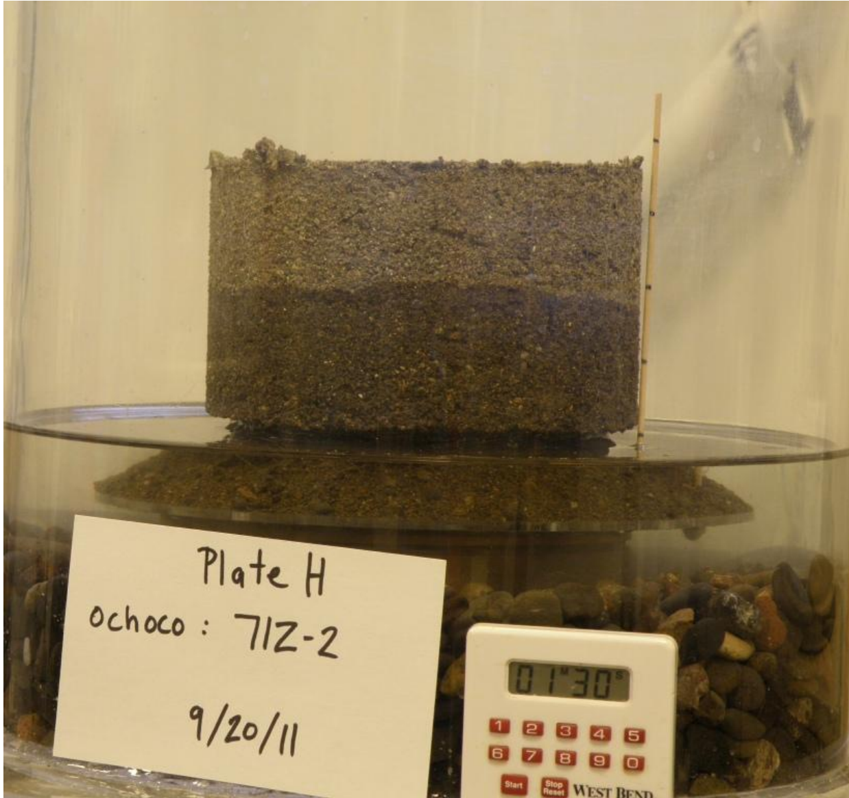
Figure A-34.—Specimen shown during the beginning of the Sand Castle Test.
