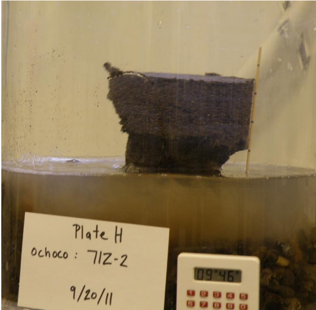
Figure A-36.—Sample shown just before failure.
