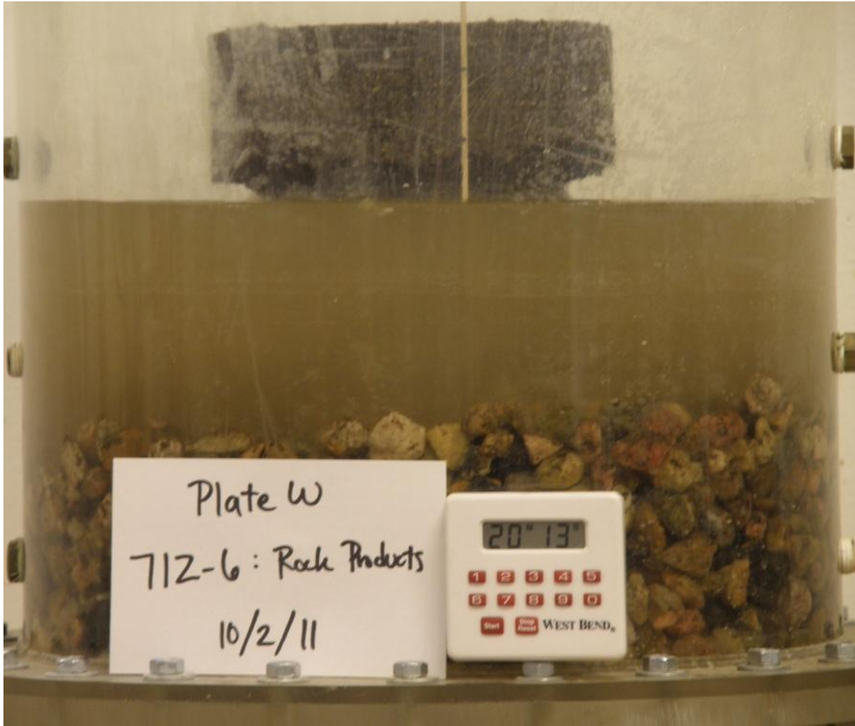
Figure A-53.—Specimen showing full absorption and 50% disintegration.
