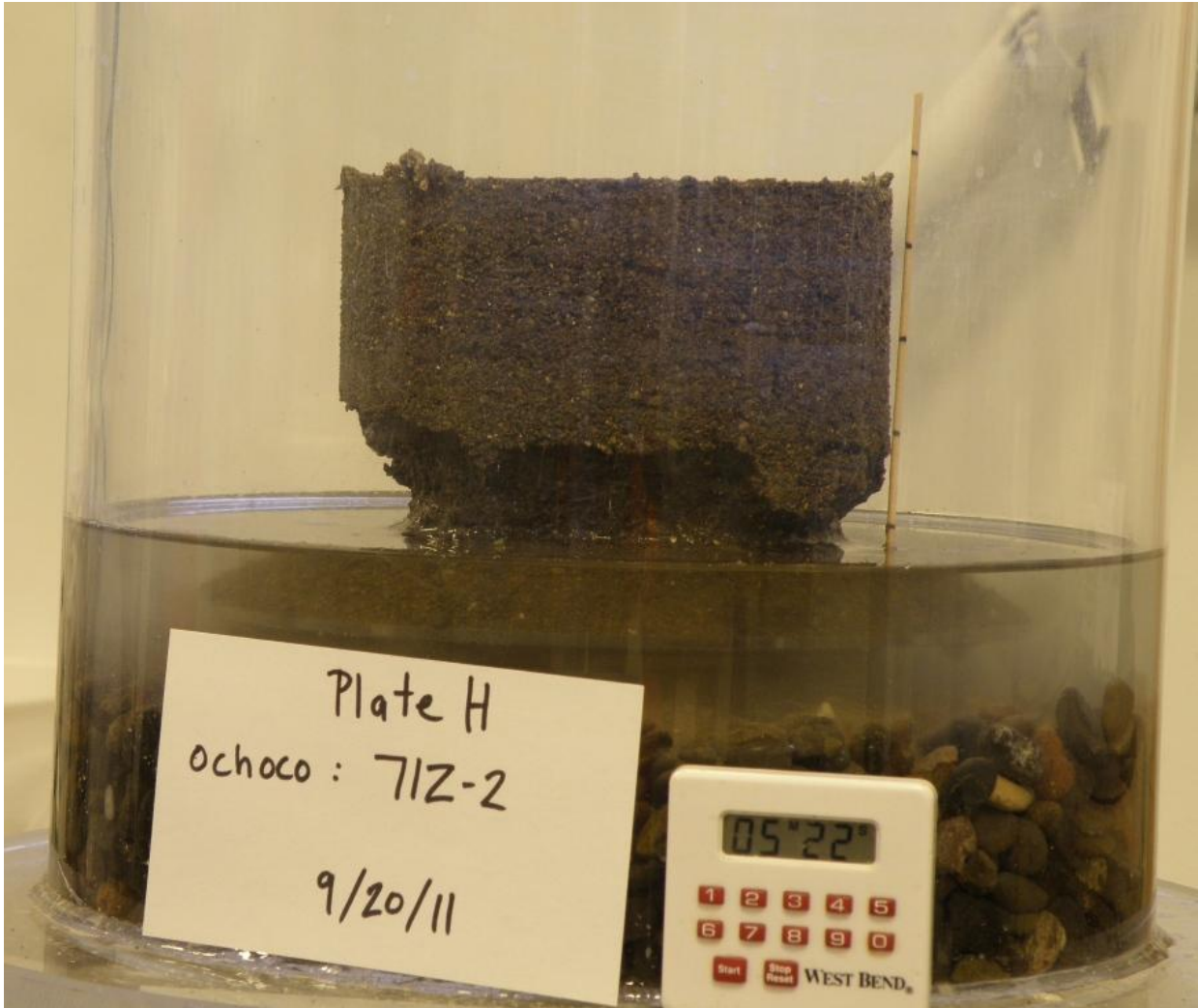
Figure A-35.—Specimen at full absorption but not yet 50% disintegration.
