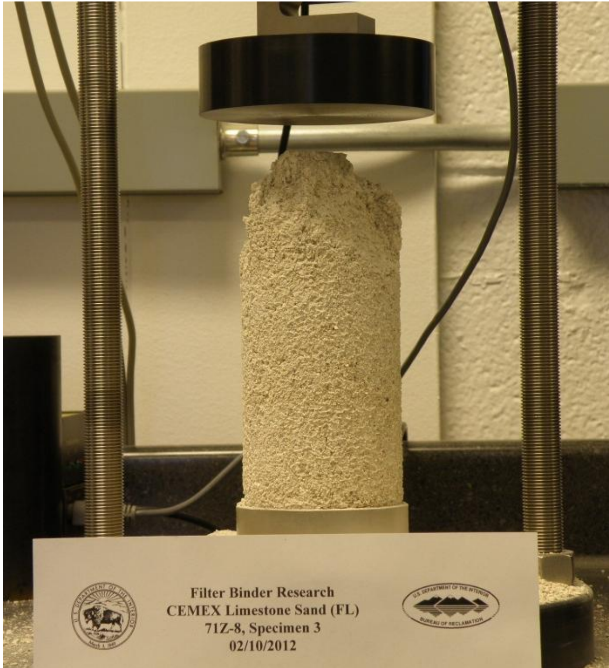
Figure A-65.—Specimen at failure.
