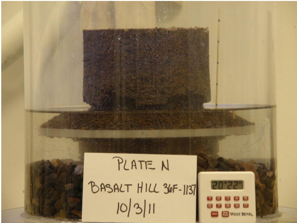
Figure A-6.—Sample has fully absorbed water, but has not reached 50% disintegration. Test has extended beyond 20 minutes.
