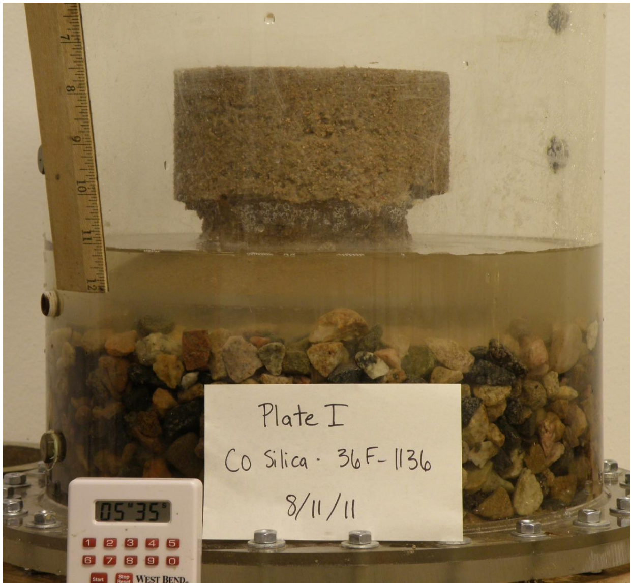
Figure A-2.—Sample has fully absorbed water and is being measured for 50% disintegration.
