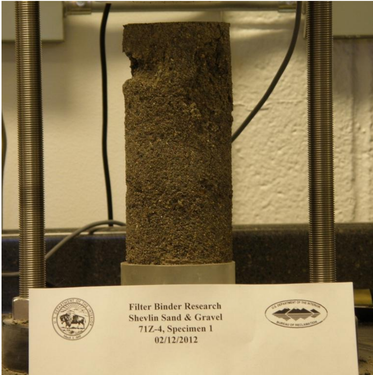
Figure A-48.—Specimen after UCS Test, showing failure.
