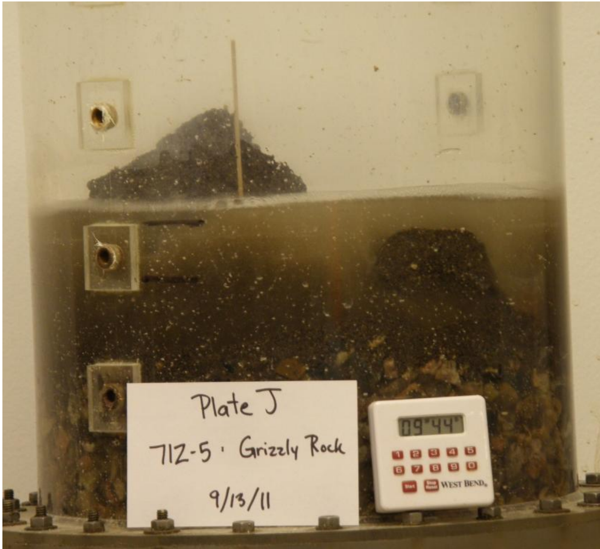
Figure A-50.—Typical specimen “topple” failure.
