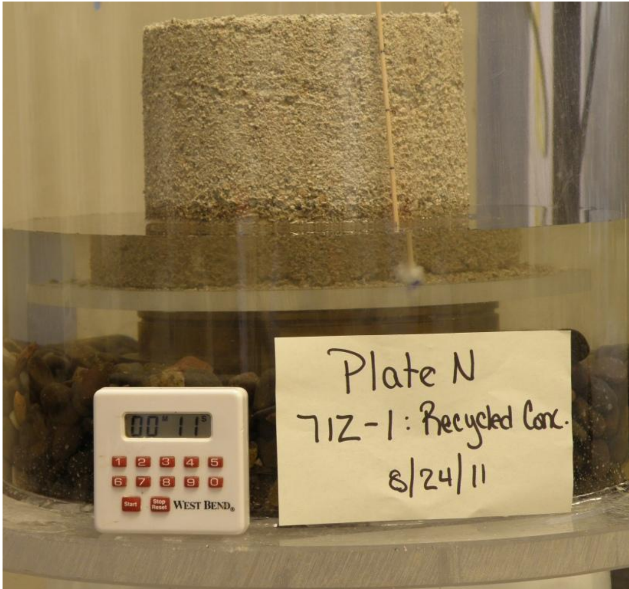
Figure A-29.—Beginning of Sand Castle Test.
