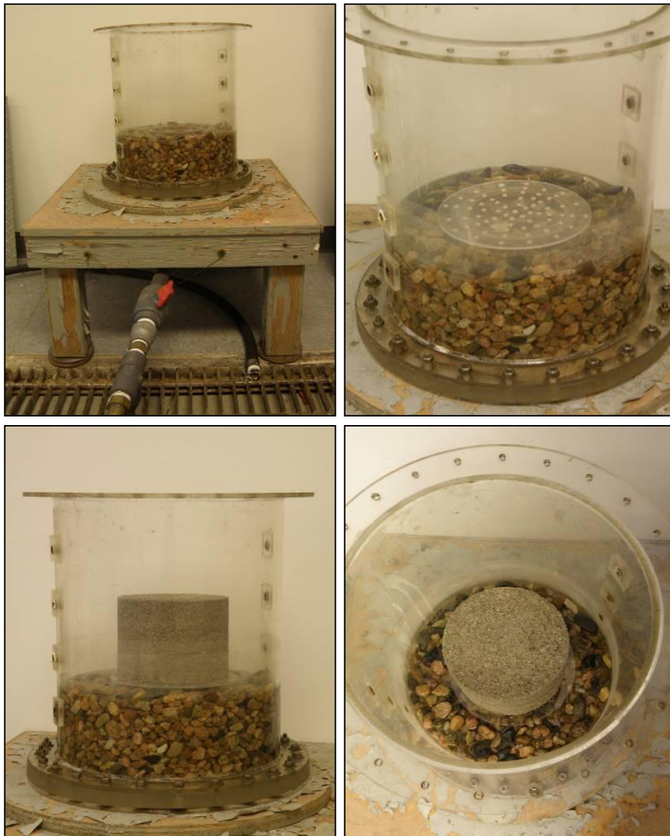
Figure 3.—Modified sand castle test apparatus.
