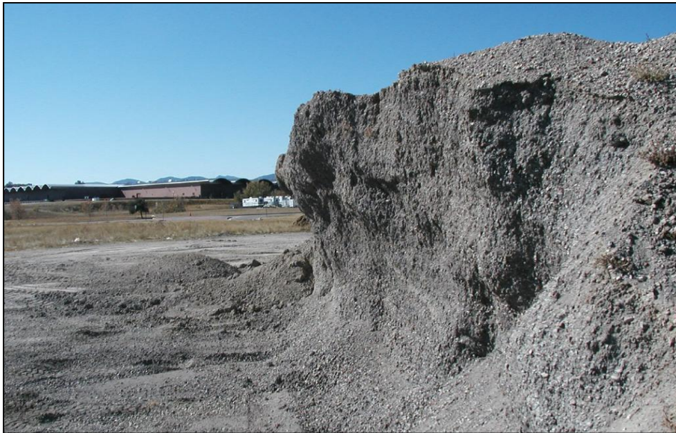
Figure 1.—Undercut recycled concrete material exhibiting cemented (cohesive) behavior.
