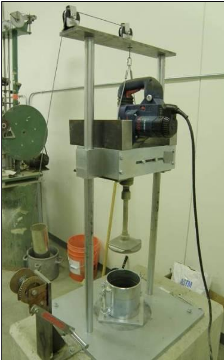
Figure 2.—Vibratory hammer compaction apparatus.
