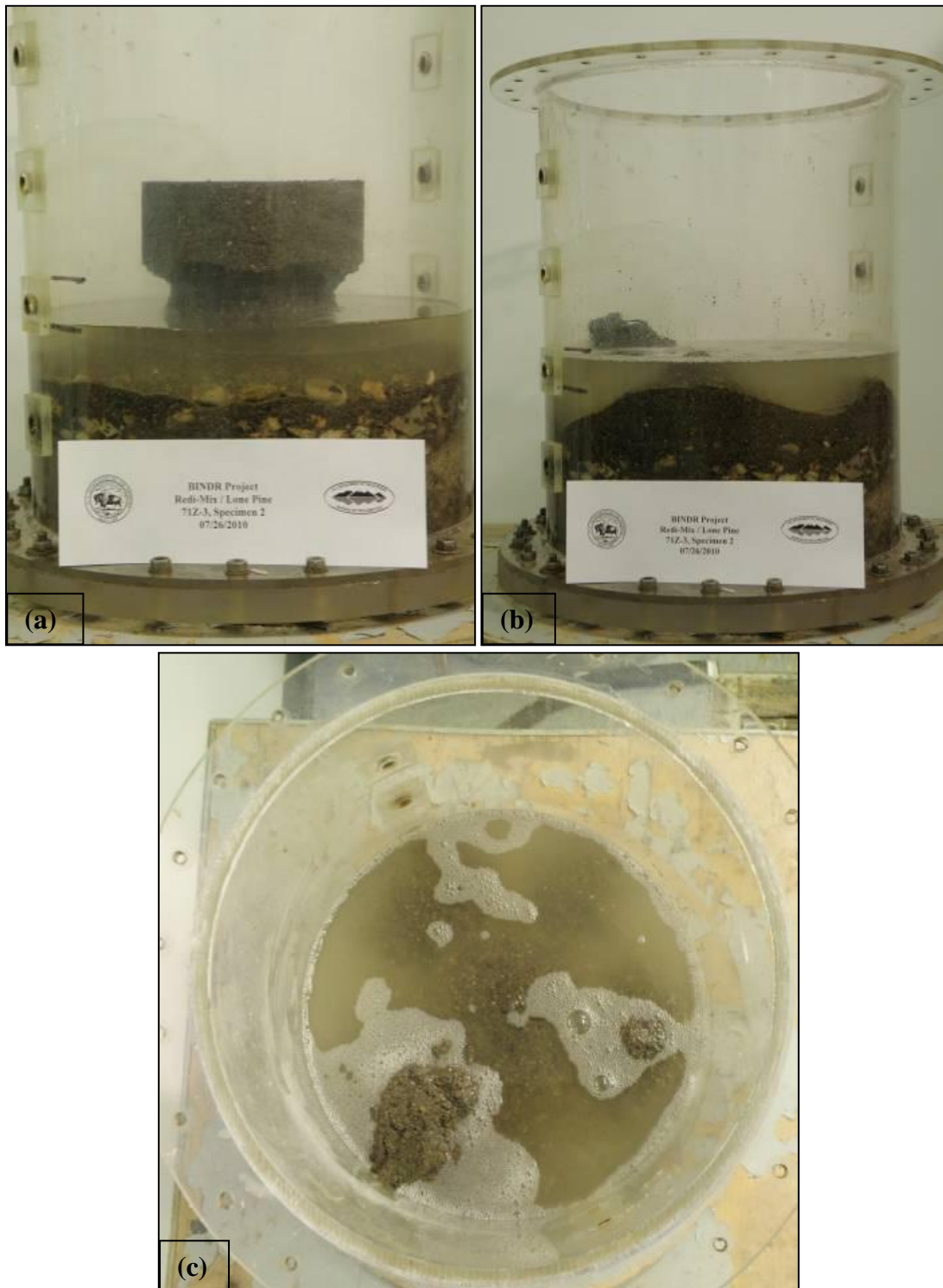
Figure 4.—Test photographs illustrating typical behavior: profile view of (a) 50 percent disintegration, (b) 100 percent disintegration, and top view of (c) 100 % disintegration.
