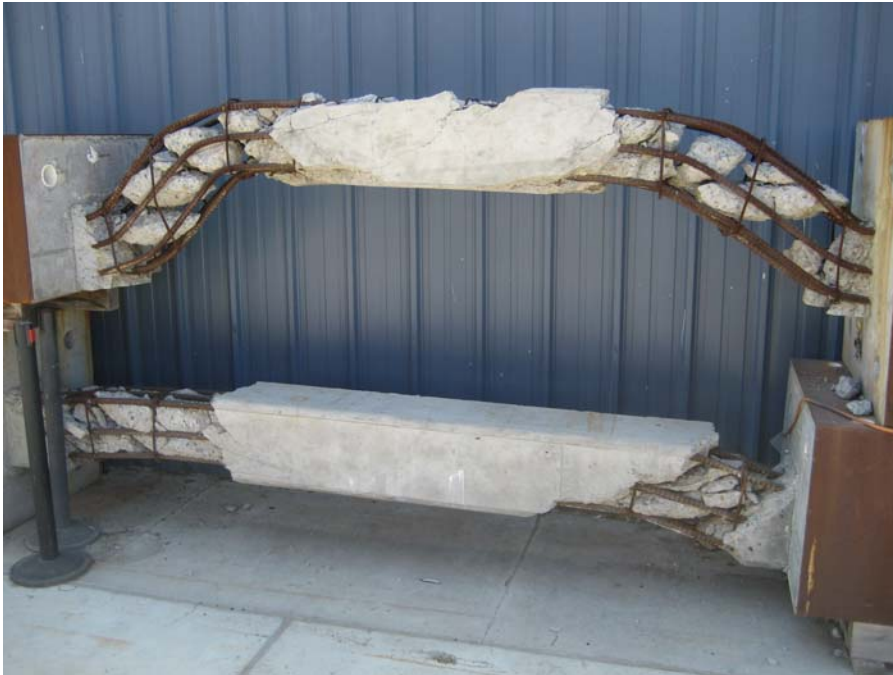
Photo 10. Damaged reinforced concrete column from previous structural testing.
