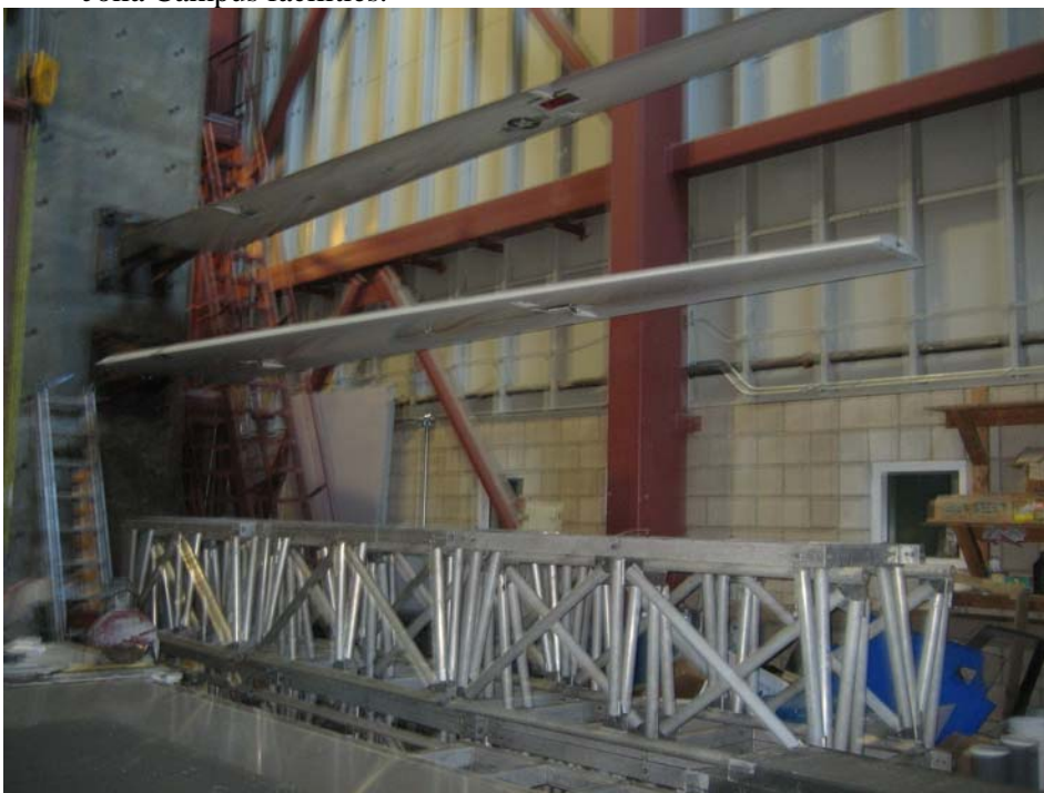
Photo 38. Composite wings of Predator remote controlled surveillance aircraft previously tested at the La Jolla Campus facilities.
