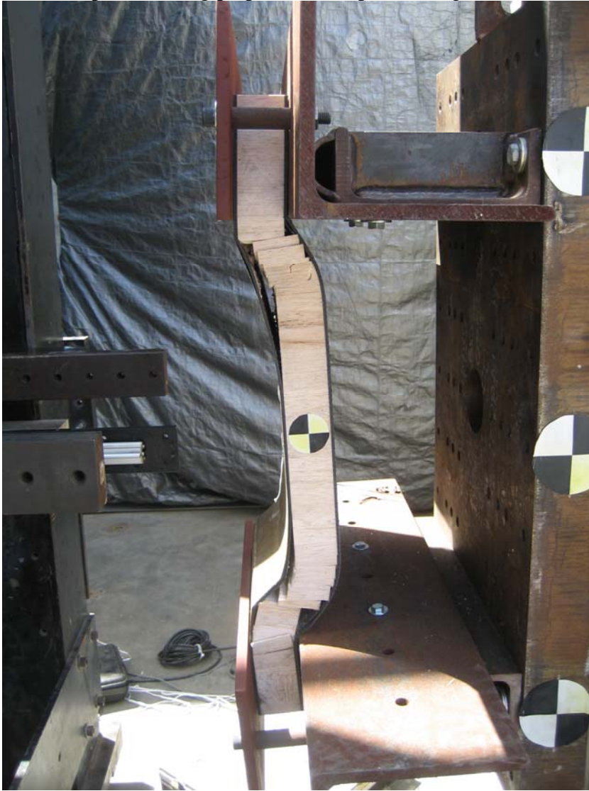
Photo 9. Composite section consisting of balsa wood between two laminar composites following impact test showing shear failure at end supports with delamination of exterior laminates. This test simulated a truck impacting a bridge pier at a scaled velocity of 20 m/sec.
