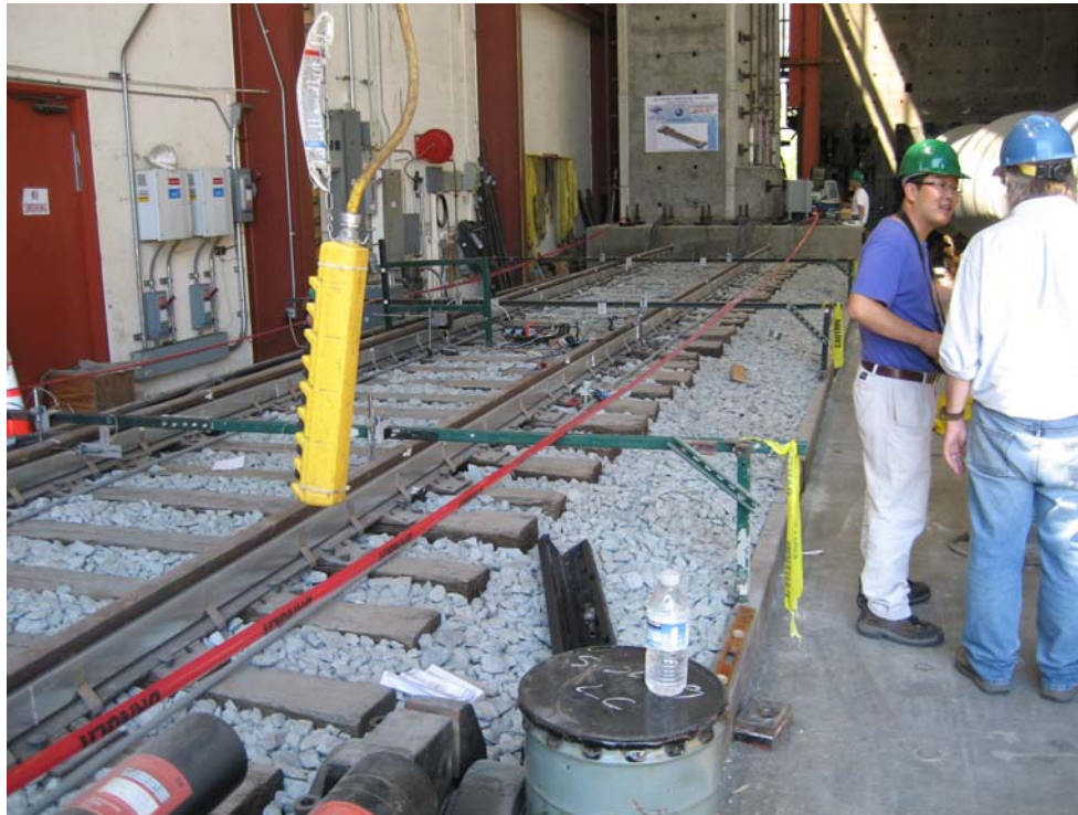
Photo 35. Railroad track at La Jolla Campus facility for non-destructive testing.
