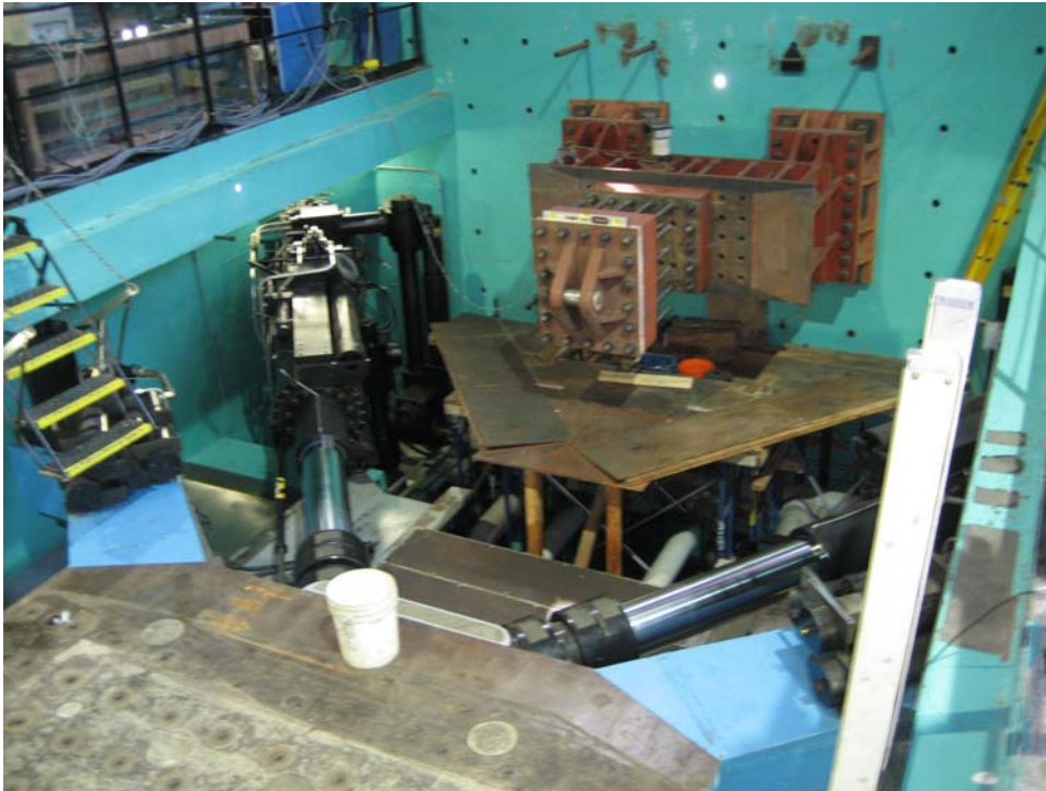
Photo 41. Structural test fixture for seismic isolation systems at the La Jolla campus facilities.
