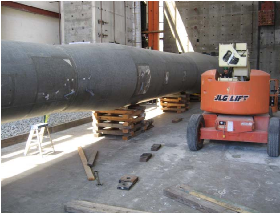
Photo 32. Wind turbine steel tower being prepared for testing at the UCSD La Jolla Campus facilities.
