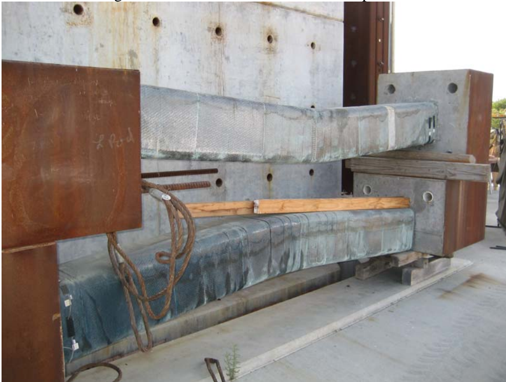
Photo 11. Composite wrapped concrete columns showing improved structural performance compared to unwrapped members shown in Photo 10.
