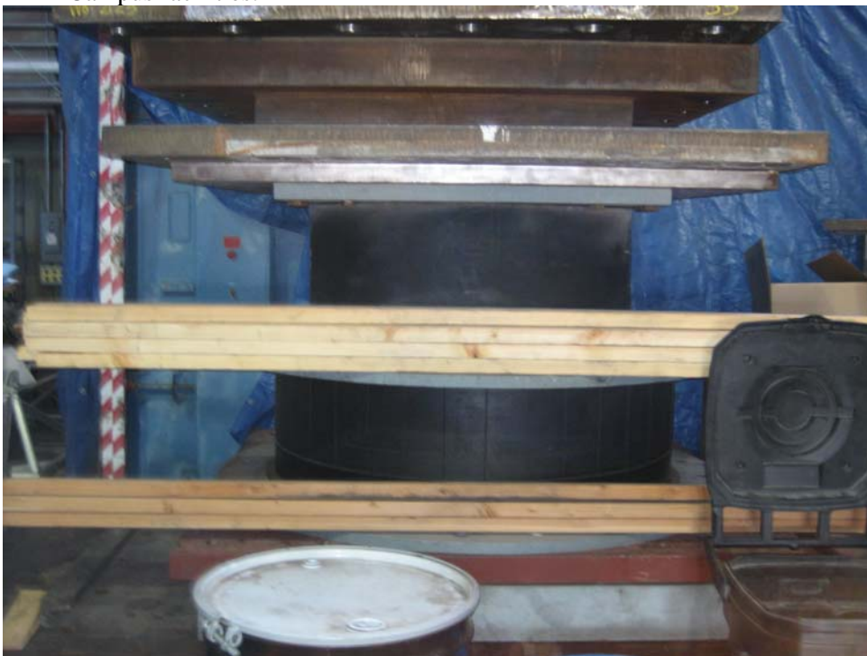
Photo 40. Structural seismic isolation system previously tested at the La Jolla Campus facilities.
