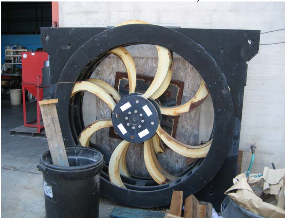
Photo 42. Structural seismic isolation system previously tested at the La Jolla Campus facilities.
