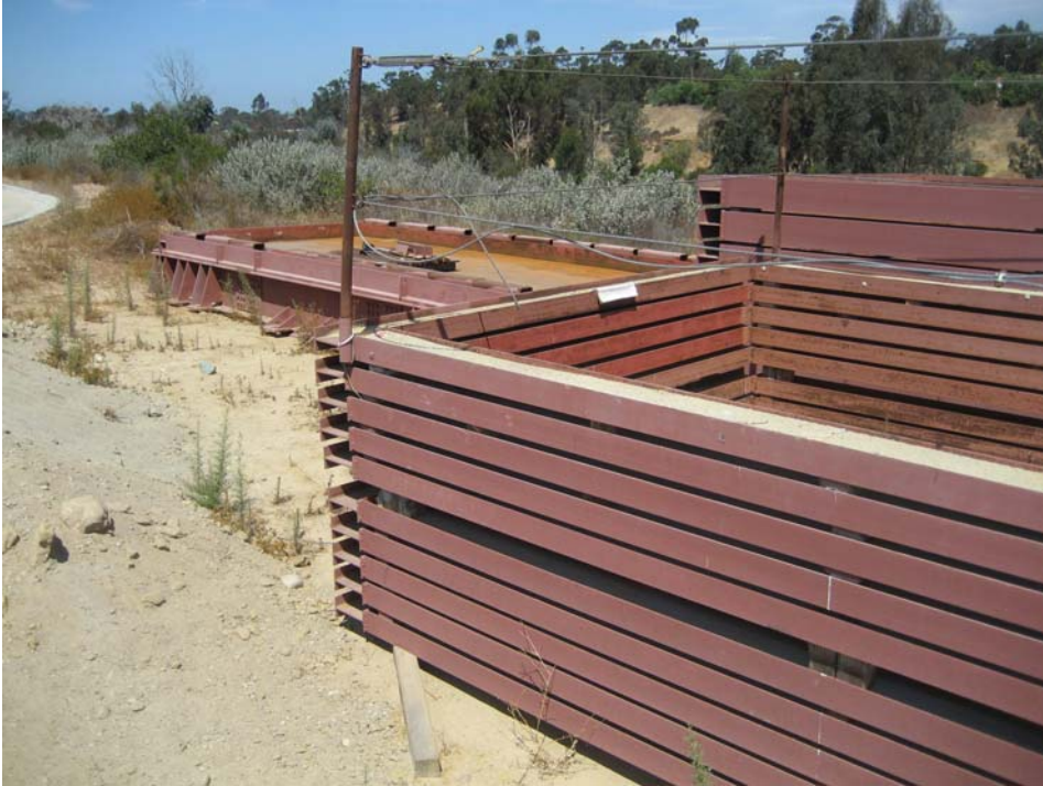
Photo 31. Laminar soil box test fixture for Patrick Wilson's large scale bridge abutment experiment.
