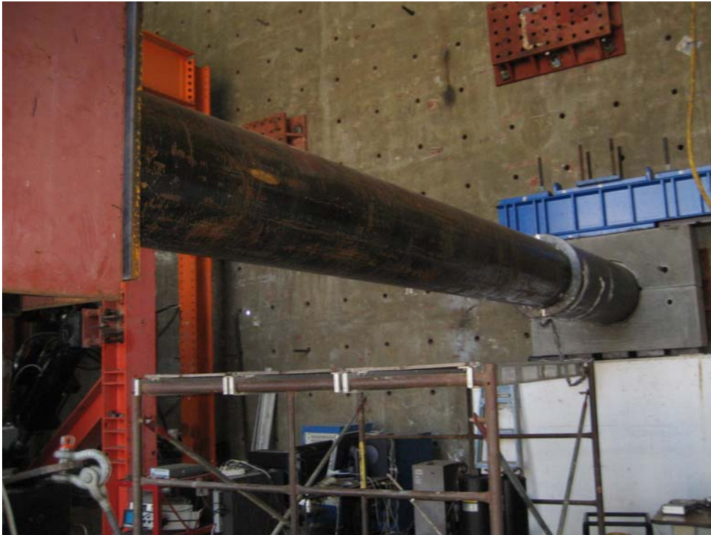
Photo 37. Structural steel highway traffic sign support column being prepared for testing at the La Jolla Campus facilities.
