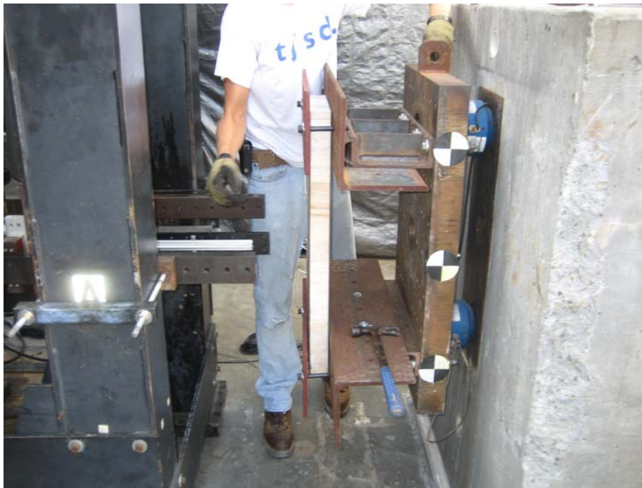
Photo 8. Composite section consisting of balsa wood between two laminar
