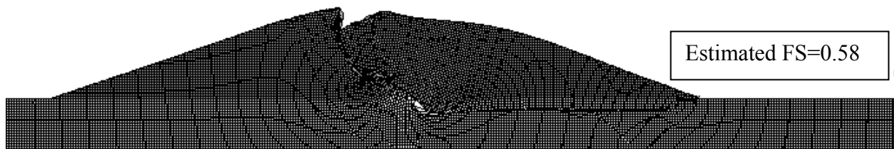
Figure 35. —DIS file showing displacement associated with the deterministic postliquefaction conditions at Ridgway Dam when the liquefiable layer is assumed to be frictionless.
