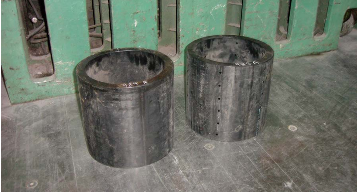
Photograph 28.—Samples of perforated and non-perforated 12-inch diameter solid-wall HDPE pressure pipe. Perforations consist of four rows of 3/8-inch holes on 2-inch centers.
