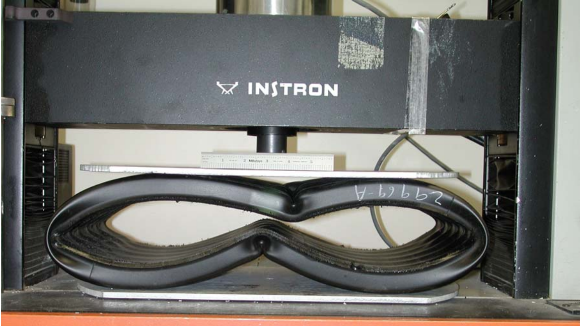
Photograph 25.—Single-wall HDPE pipe – “binocular” failure mode.
