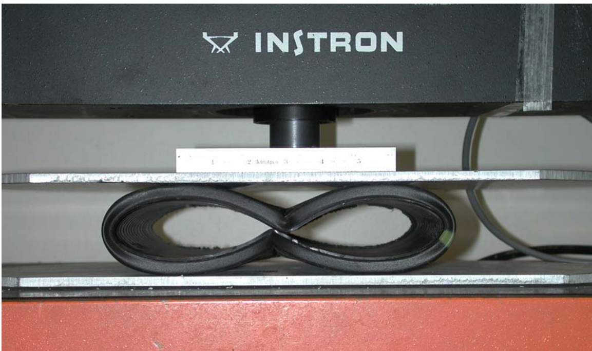
Photograph 20.—“Binocular” failure mode.
