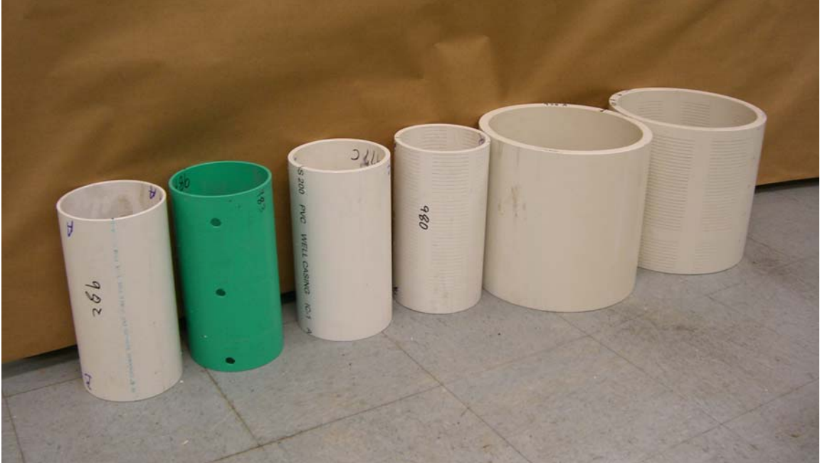
Photograph 9.—PVC solid-wall drainpipe and pressure pipe in 6- and 12-inch diameters.
