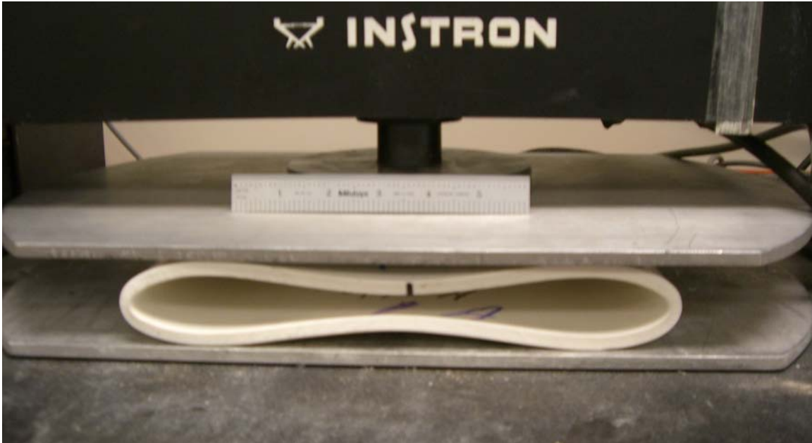
Photograph 13.—Pancake failure mode for thin-walled PVC drainpipe.
