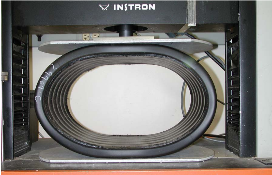
Photograph 23.—Pipe walls begin to buckle at approximately 40 percent deflection (maximum load).
