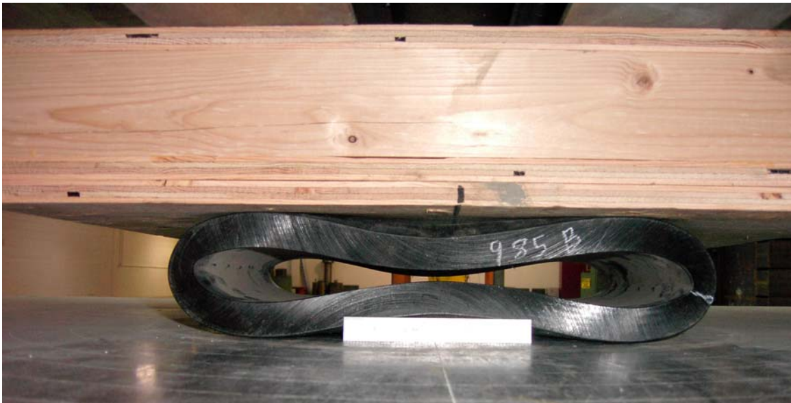
Photograph 31.—Pancake failure mode – slightly binocular.
