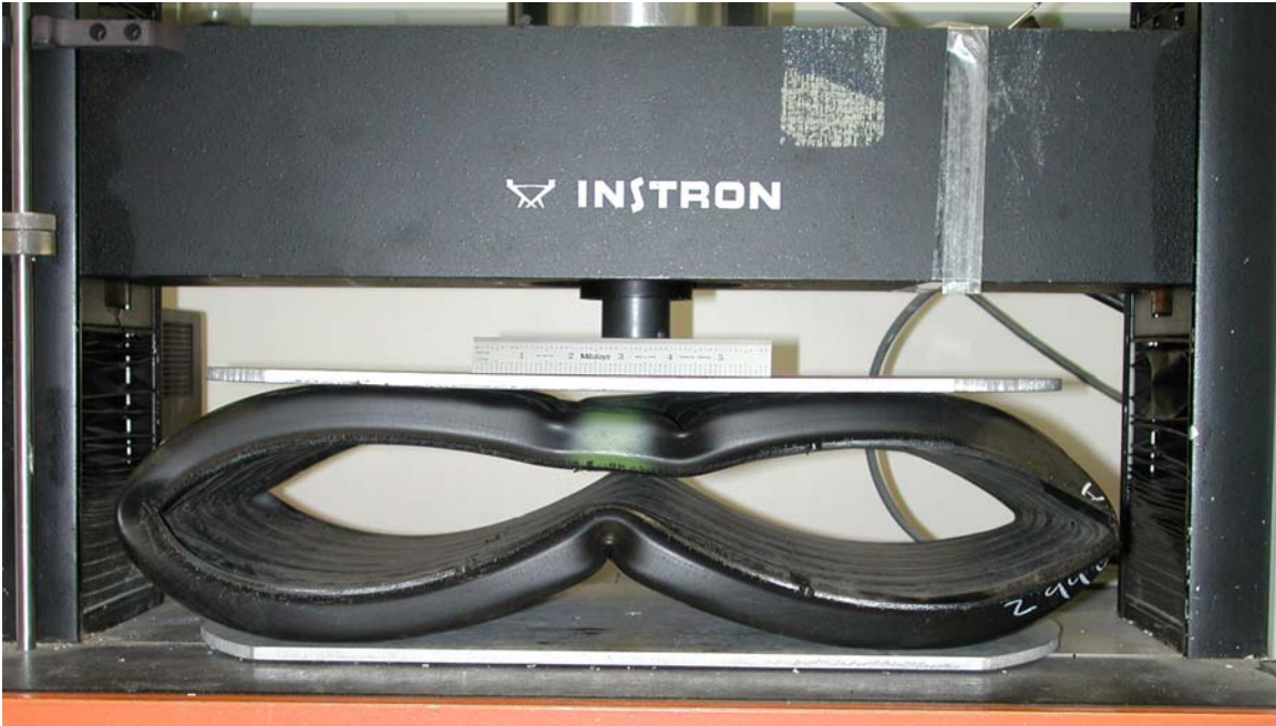
Photograph 26.—Single-wall pipe – “inverted heart” failure mode.
