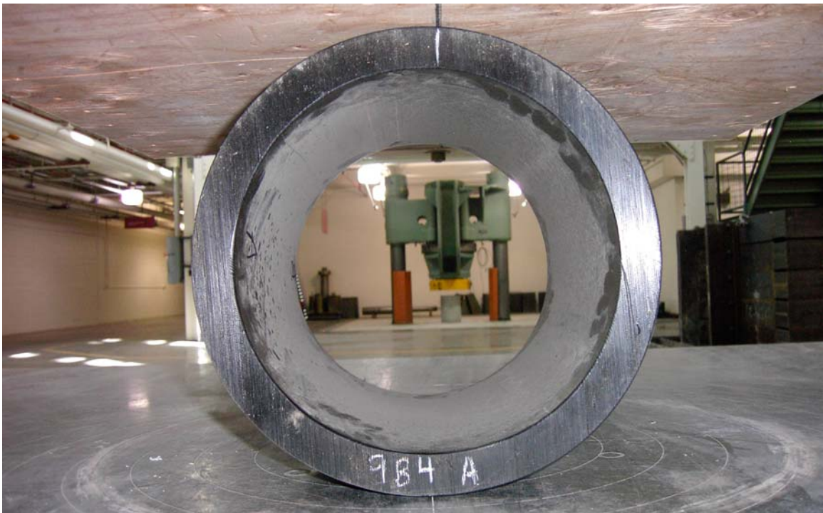
Photograph 29.—HDPE solid-wall ready for testing.
