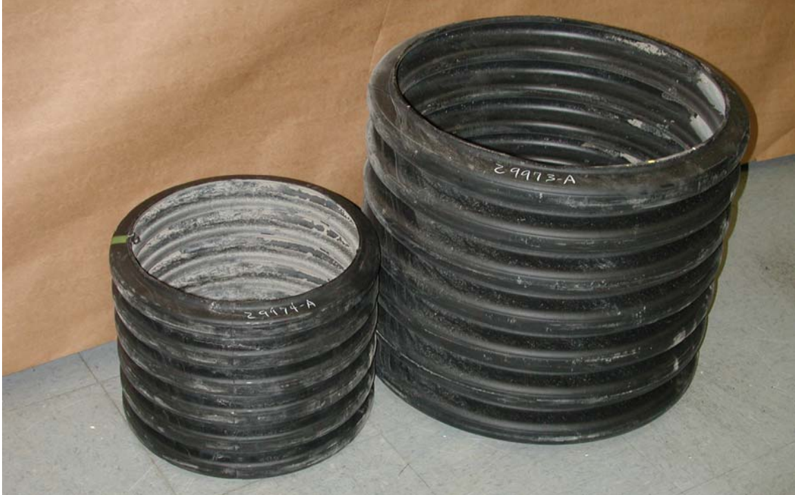
Photograph 21.—Samples of single-wall corrugated HDPE drainpipe include 12- and 18-inch diameter (perforated and non-perforated).
