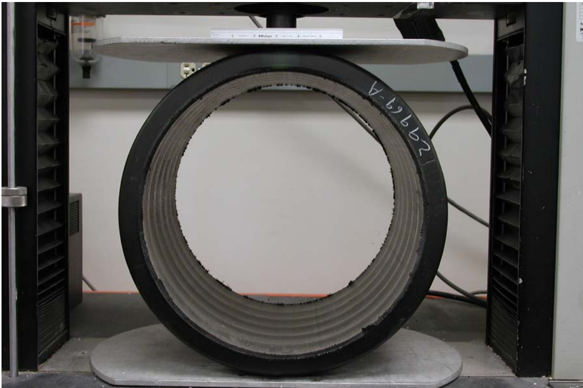
Photograph 16.—Double-wall HDPE pipe at 0 (zero) percent deflection.
