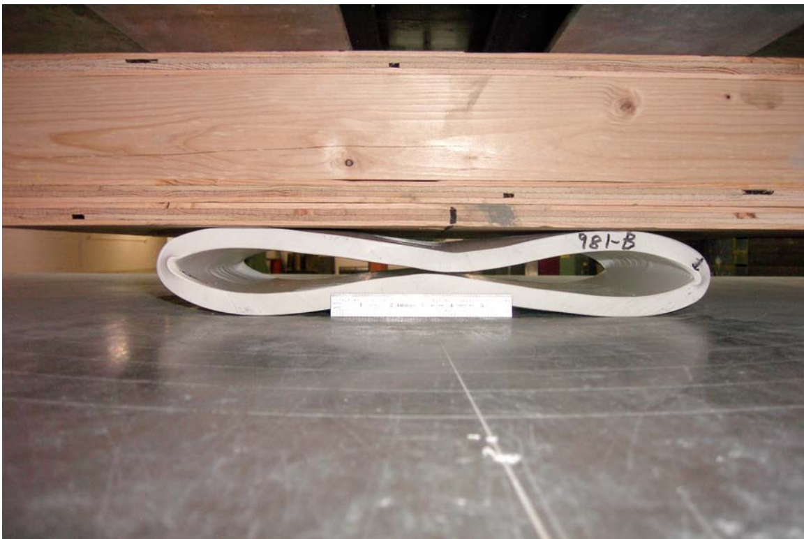
Photograph 14.—Pancake failure mode for sample of PVC pressure pipe.
