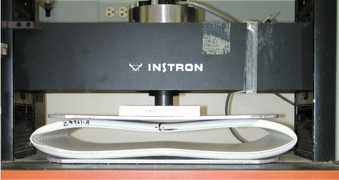
Photograph 5.—Pancake failure mode.
