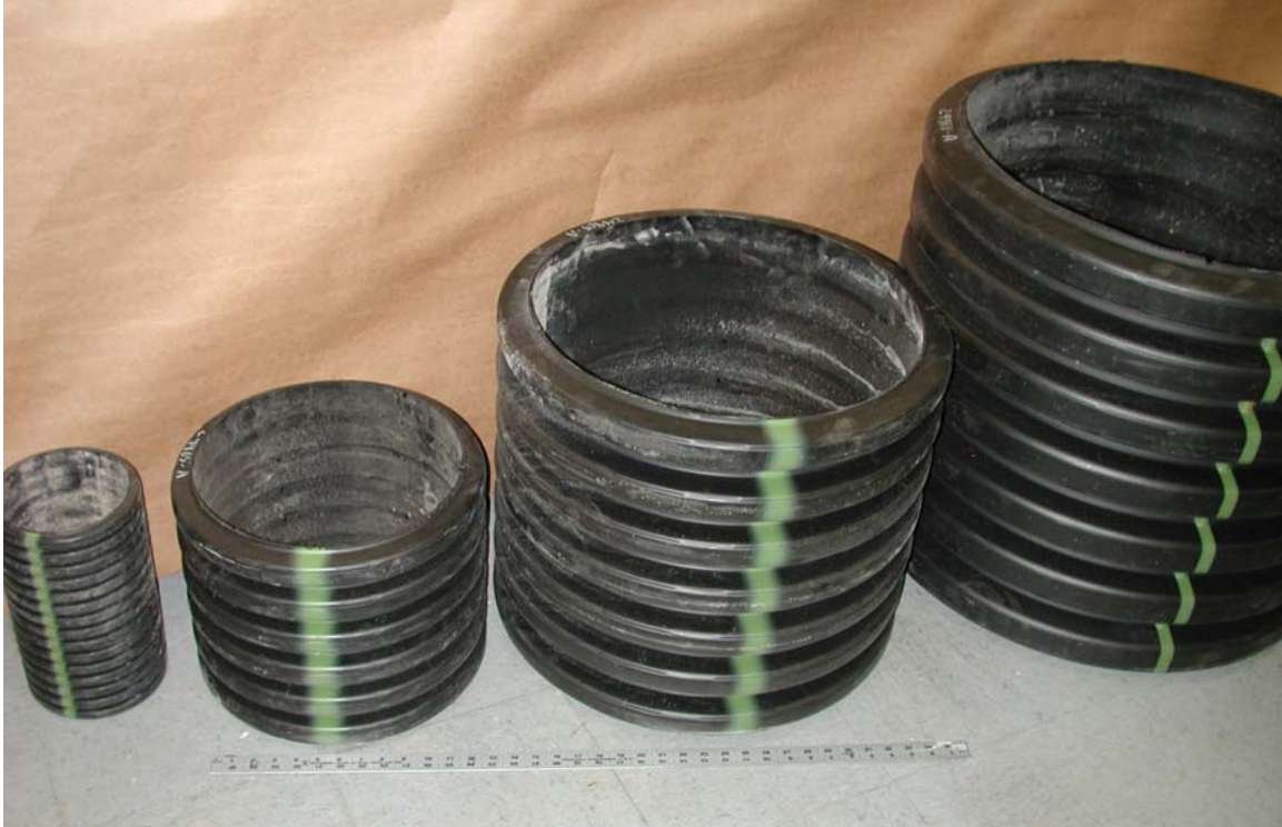
Photograph 15.—Samples of HDPE perforated and non-perforated double-wall corrugated drainpipe, including 6-, 12-, 18-, and 24-inch diameter.
