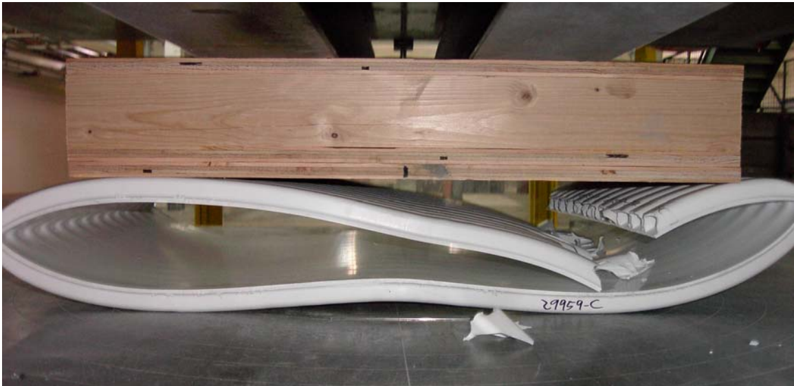
Photograph 8.—Pancake failure mode with shattered pipe wall.
