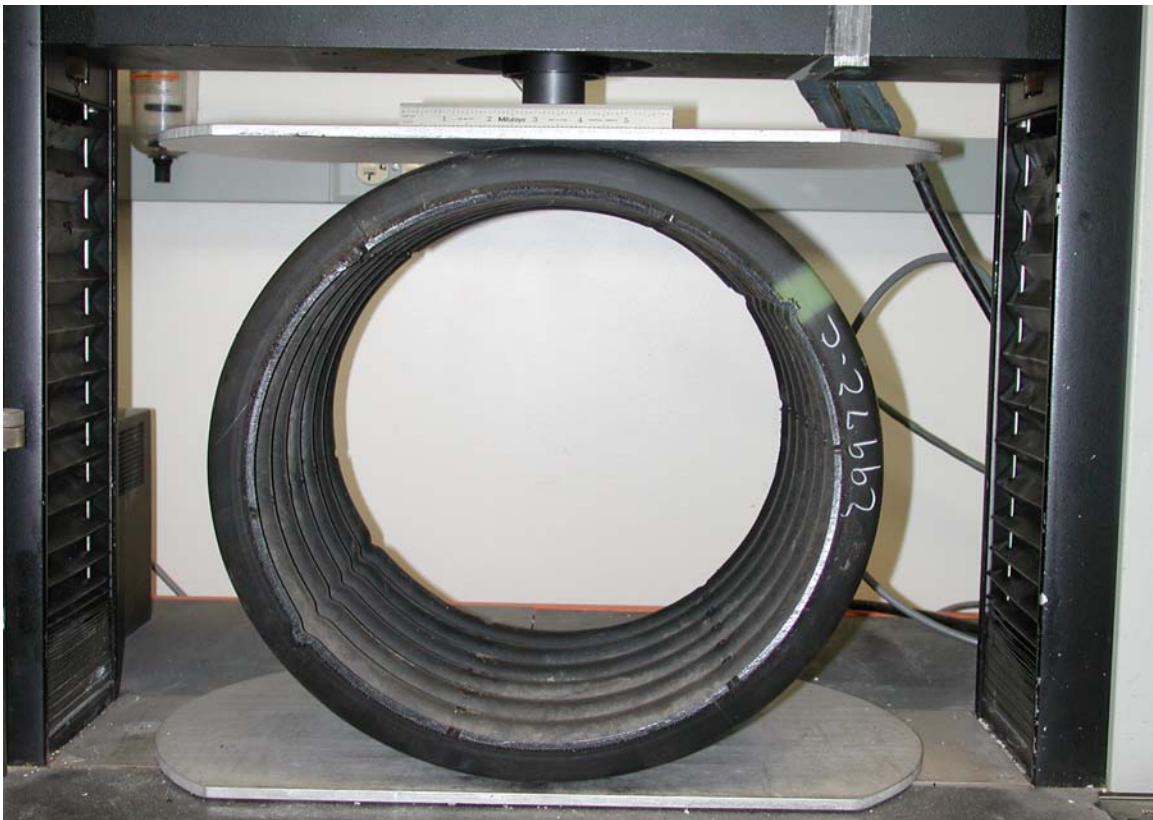
Photograph 22.—12-inch diameter sample loaded in the test machine and ready for testing.
