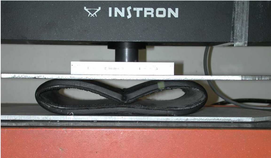
Photograph 19.—“Heart” failure mode.
