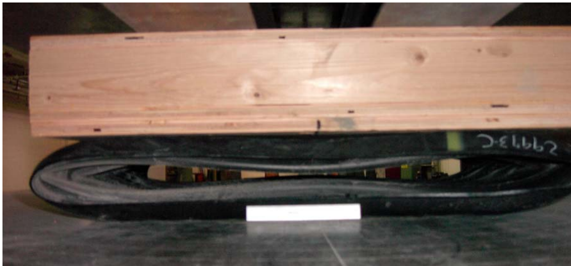
Photograph 27.—Pancake failure mode.
