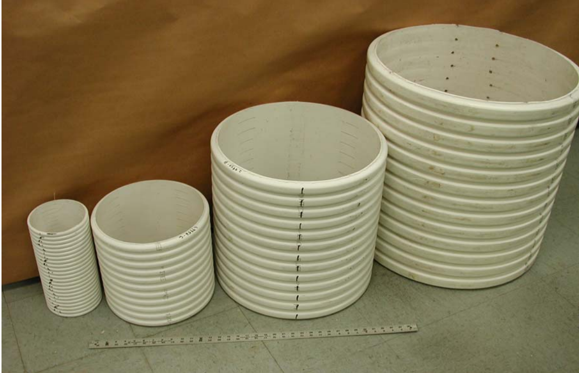
Photograph 1.—Corrugated double-wall PVC pipe, 6-, 12-, 18-, and 24-inch diameter.
