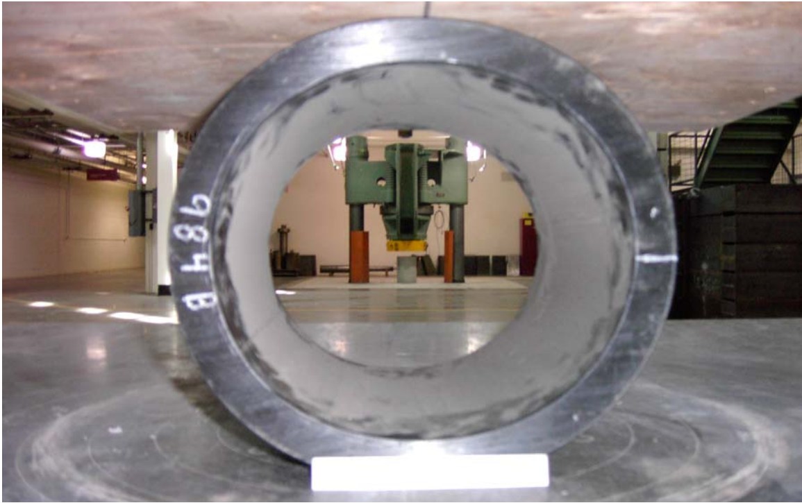
Photograph 30.—Pipe at 5 percent deflection.
