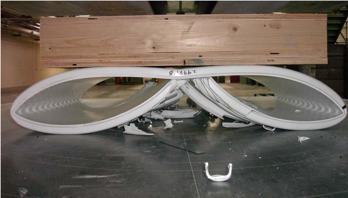
Photograph 6.—Shattered pipe wall with inverted heart failure mode.
