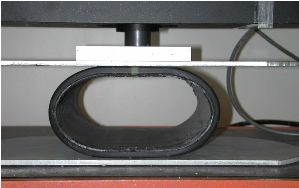
Photograph 18.—HDPE pipe at maximum load – buckling of pipe wall at approximately 40 percent deflection.
