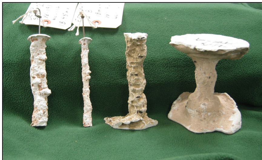
Figure 6. —Plaster casts of eroded holes illustrate difficulties in measuring final hole diameter following an HET.
