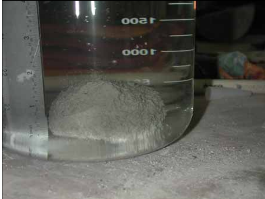
Figure 12. —Sample of mortar with a flow of 25 placed in standing water.
