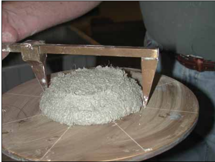
Figure 8. —Mortar flow consistency test: flow is 25 after 25 drops on the flow table indicating a 25-percent increase in diameter.
