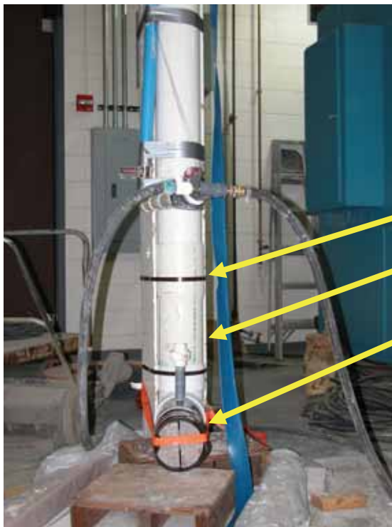
Figure 1. —Underwater crack test standpipe assembly with cracked concrete cylinder.
