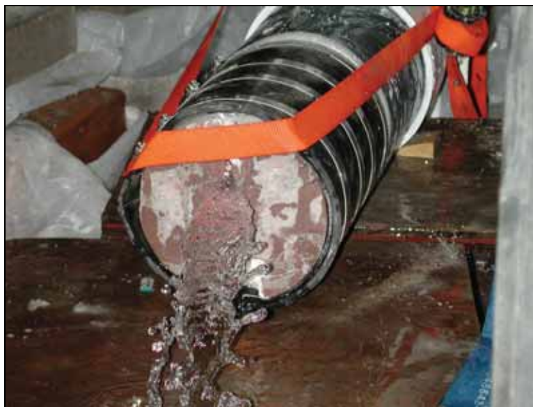
Figure 3. —End view of water flow through a cracked concrete test specimen under 3 m (10 ft) of hydraulic head before mortar injection. Flow is about 40 L/min (10 gal/min).
