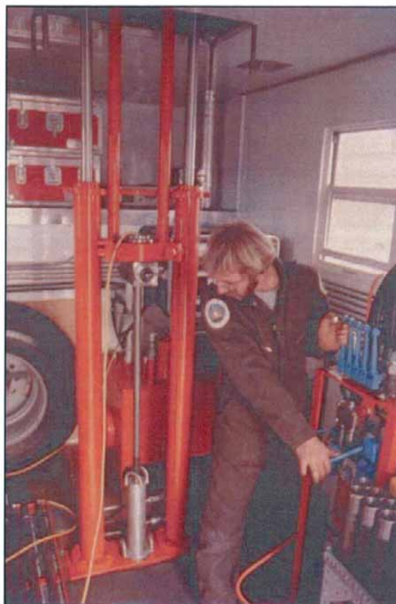
Figure 9. —Hydraulic CPT pushing mechanism.
