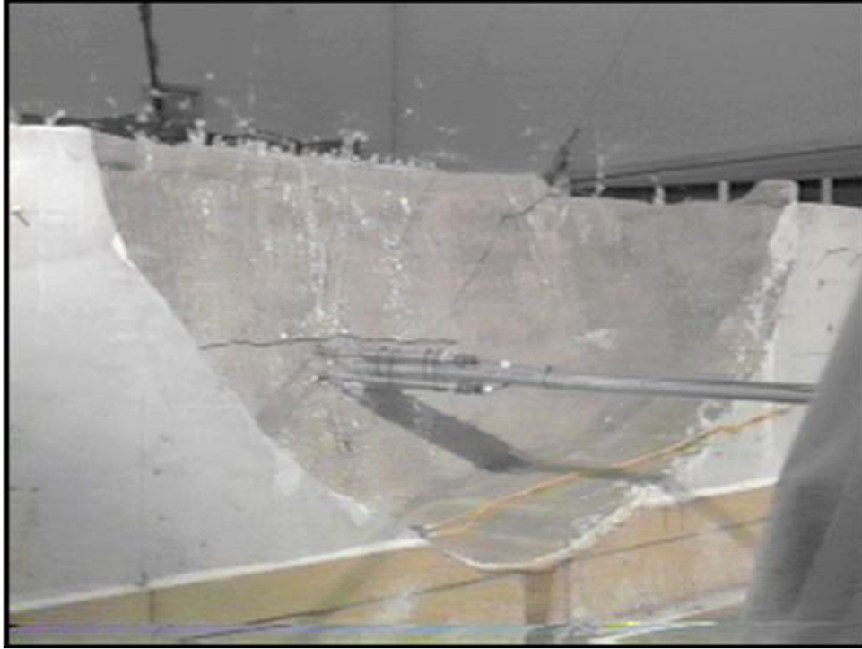
Figure 29a. —Model 10—horizontal joint initial failure, south camera.
