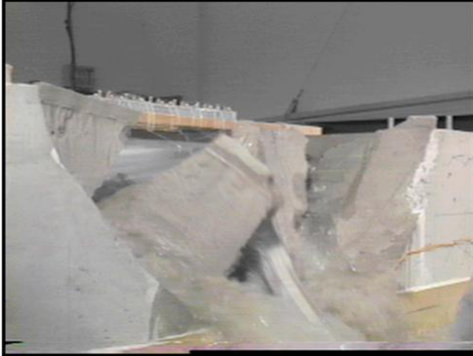
Figure 30a. —Model 11—vertical joint south view, final failure.
