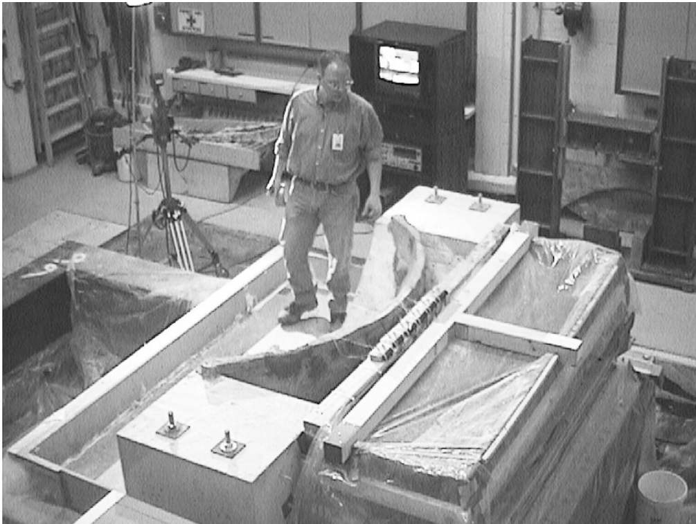
Figure 4 - Shake table model ready for testing, note reservoir behind dam (covered in plastic)
