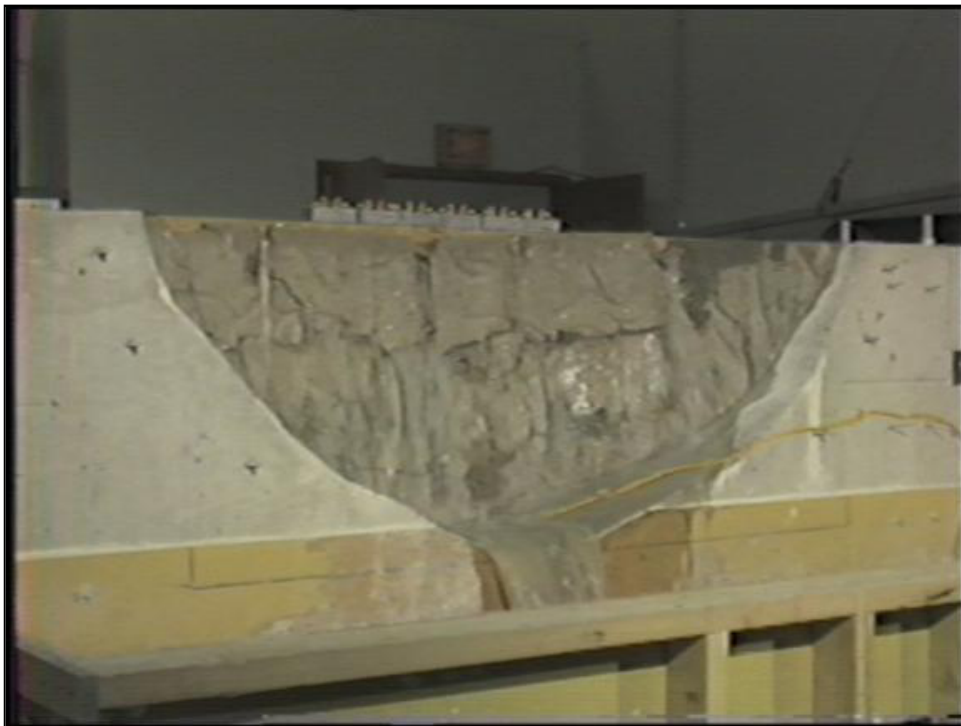
Figure 31b. —Model 11—vertical joint south view, final failure.
