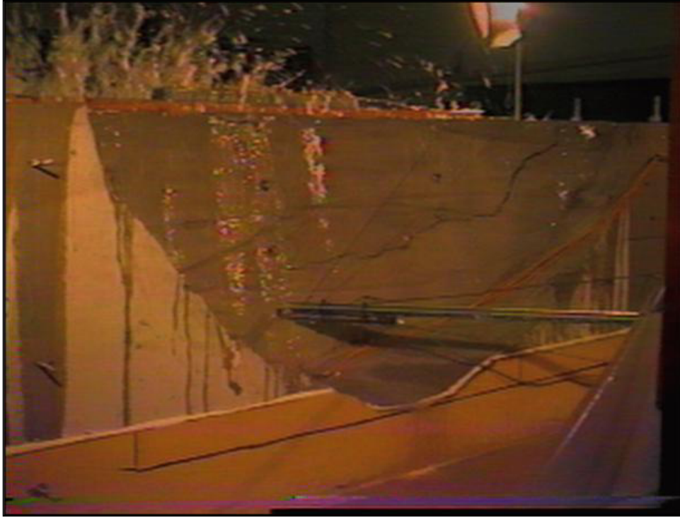
Figure 28a. —Monolithic model 2 initial cracking.
