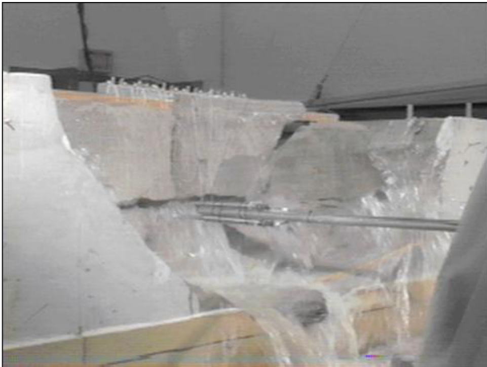
Figure 29b. —Model 10—horizontal joint final failure.
