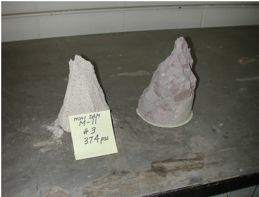
Figure 1 - Failure of Modeled Material and 50 Year recovered Core
