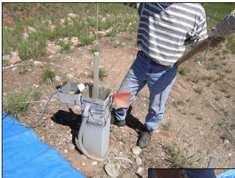
2.2 Lowering the bailer into the well.
