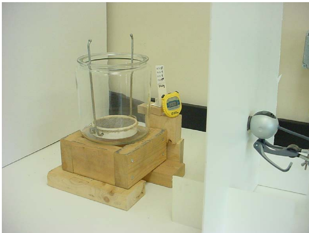
Figure 7.2 Test configuration for Sand Castle Test
