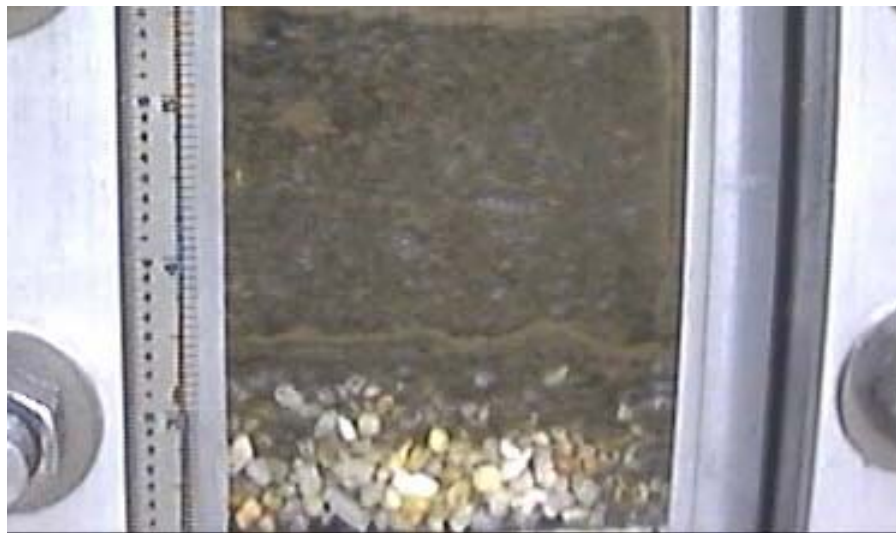
Figure 5.12 Clogging layer after Test 5
