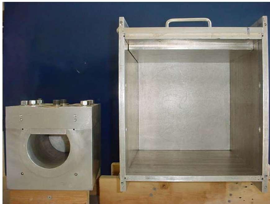
Figure 6.2 Comparison of cross section of the two filter test device
