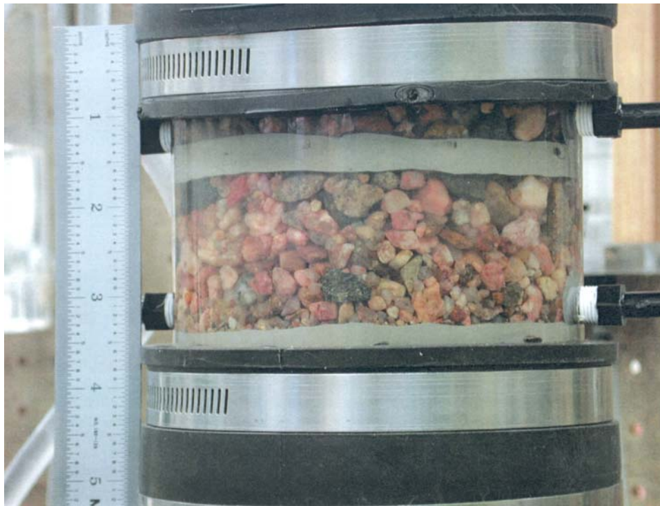
Figure 2.—Close-up of test permeameter with gravel envelope. Clay seals prevent vertical flow along the permeameter wall.
