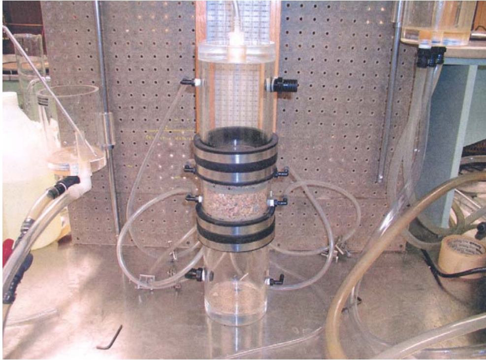
Figure 1.—Permeameter test device (modified Gradient Ratio).
