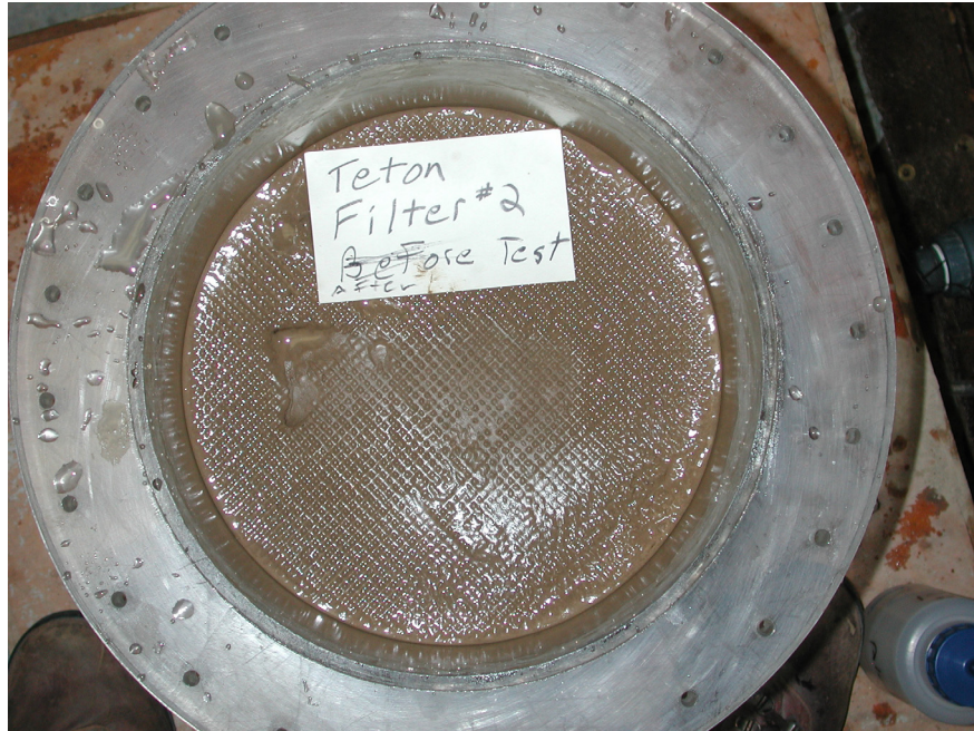
Photo 1 – NEF Test, Teton Material, Filter #2
