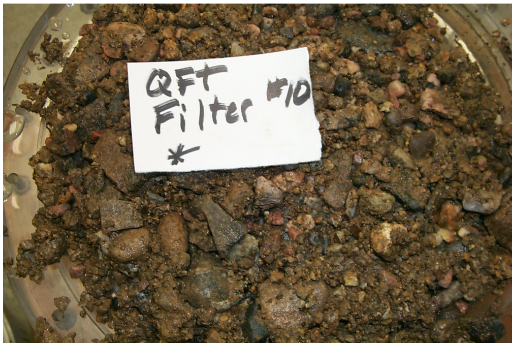
Photo 8 – CEF Test, Keechelus Material, Filter #10 (Bottom of Base Material)
