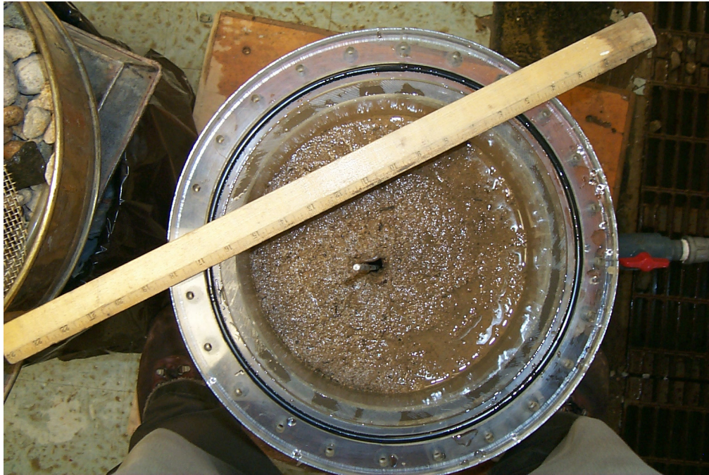
Photo 9 – CEF Test, Keechelus Material, Filter #11
