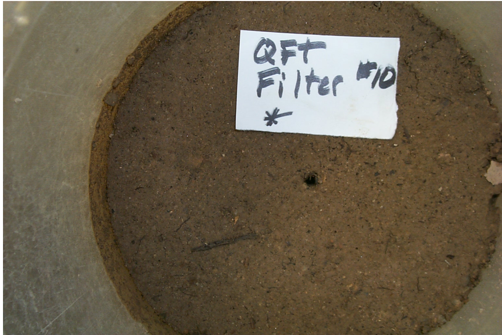
Photo 7 – CEF Test, Keechelus Material, Filter #10 (Top of Base Material)
