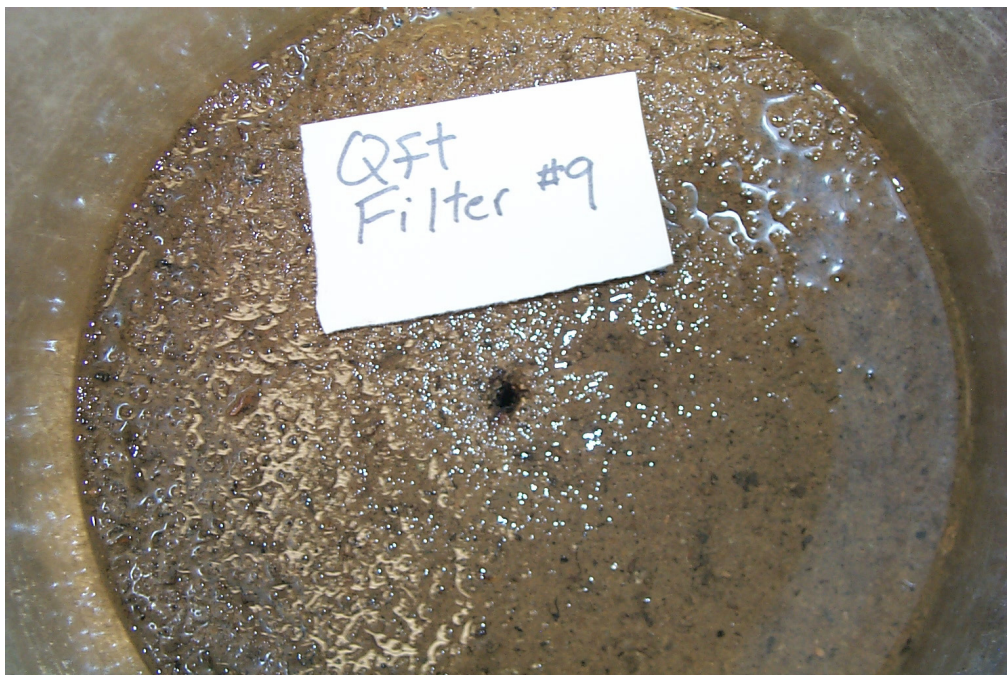
Photo 6 – CEF Test, Keechelus Material, Filter #9
