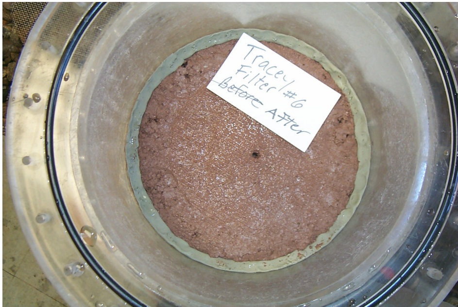
Photo 6 – CEF Test, Tracey Material, Filter #6
