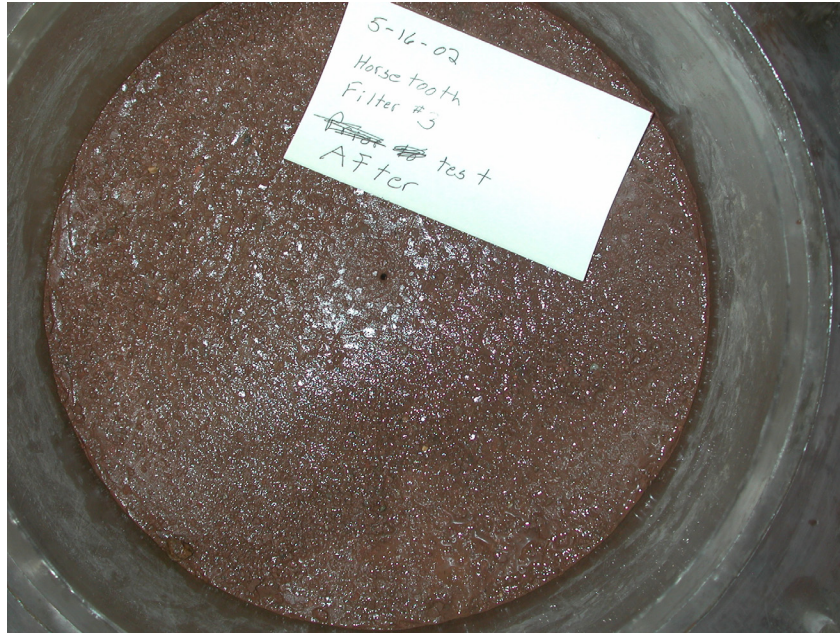
Photo 1 – NEF Test, Horsetooth Material, Filter #3
