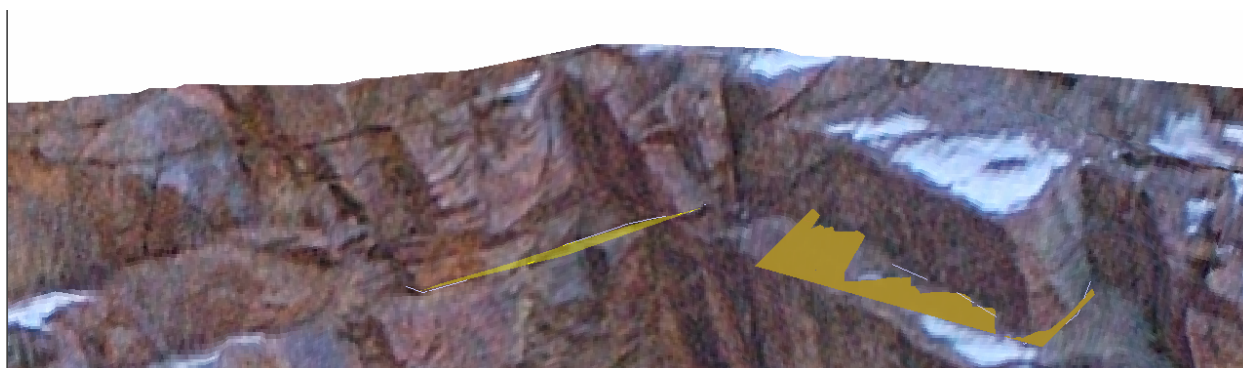
Figure 14.—Using two traces (and planes) to improve the mapping of the actual joints.
