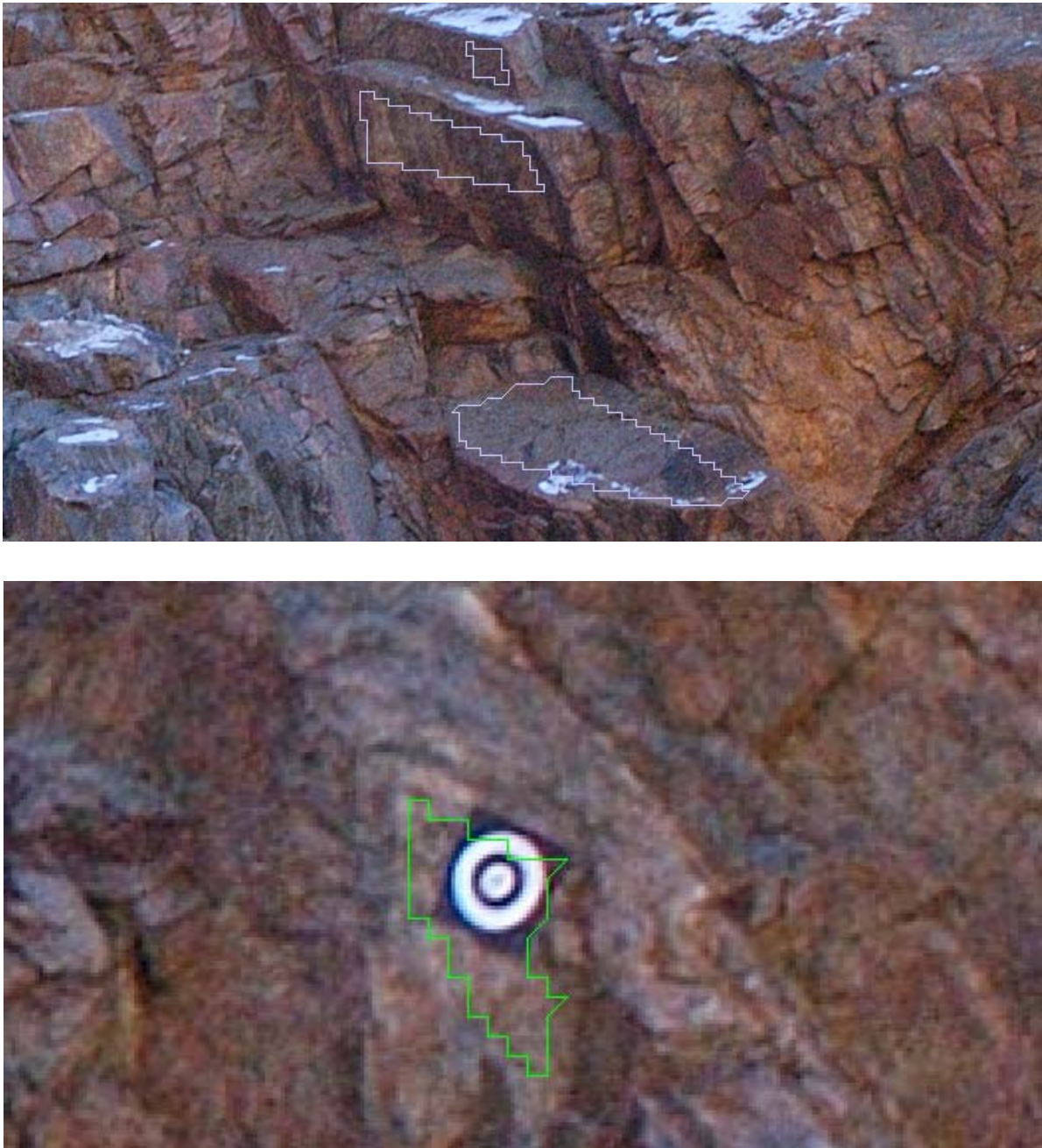
Figure 6.—Polygon drawing objects used to map the orientations of several block faces.
