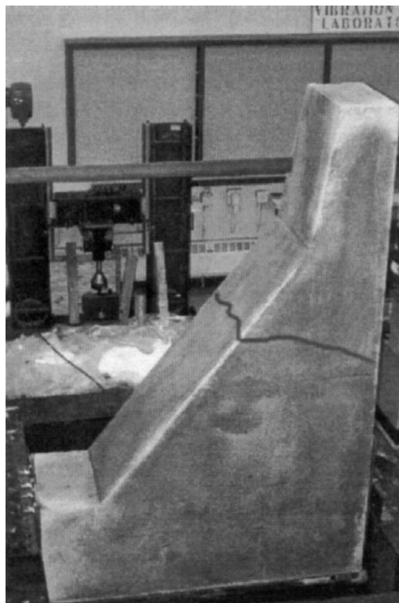
Figure 5.—First Koyana model mounted on the shake table. The shrinkage crack and eventual failure plane is sketched in.
