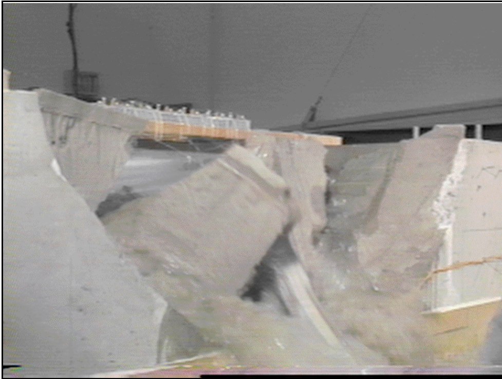
Figure 30a.—Model 11 - vertical joint south view, final failure.
