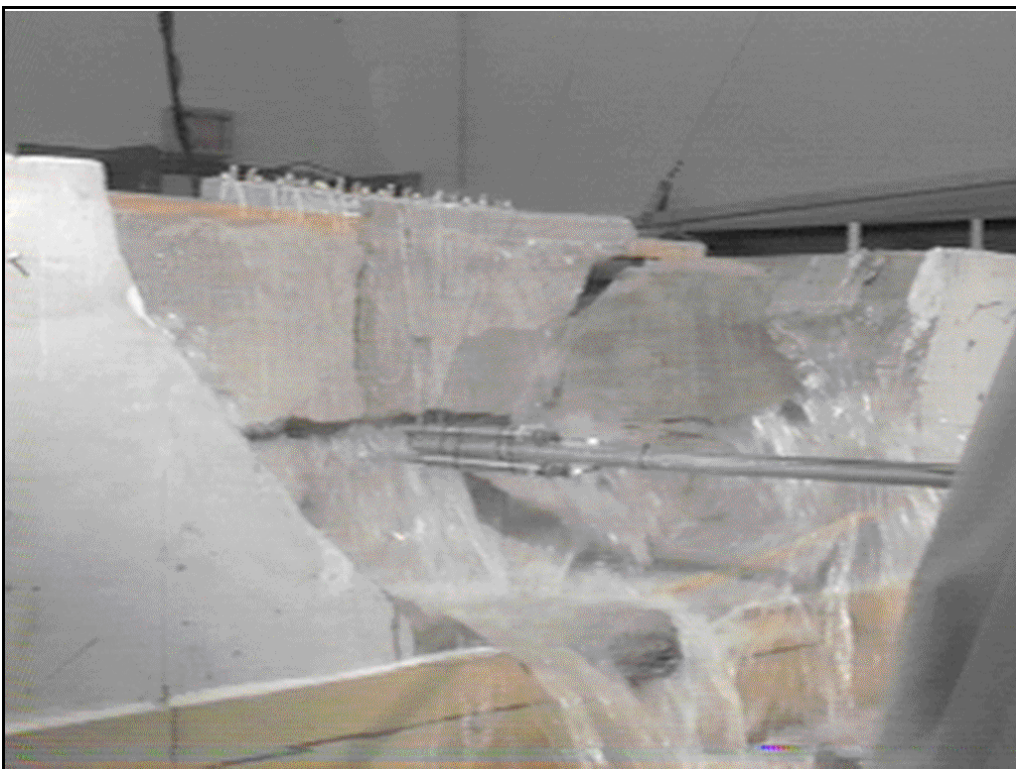
Figure 29b.—Model 10 - horizontal joint final failure.
