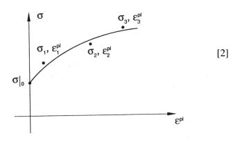
When Stabilized Cycle Data is used to define the kinematic hardening component, tabulated values of stress and strain from the stabilized cycle of a specimen that has been subjected to symmetric strain cycles are required. A stabilized cycle is obtained by cycling the specimen over a fixed strain range until a steady-state condition is reached. A stabilized cycle is illustrated in the following figure.
