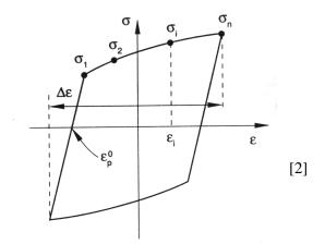
When the direct parameters method is used to define the kinematic hardening component, the following material parameters are entered directly.
