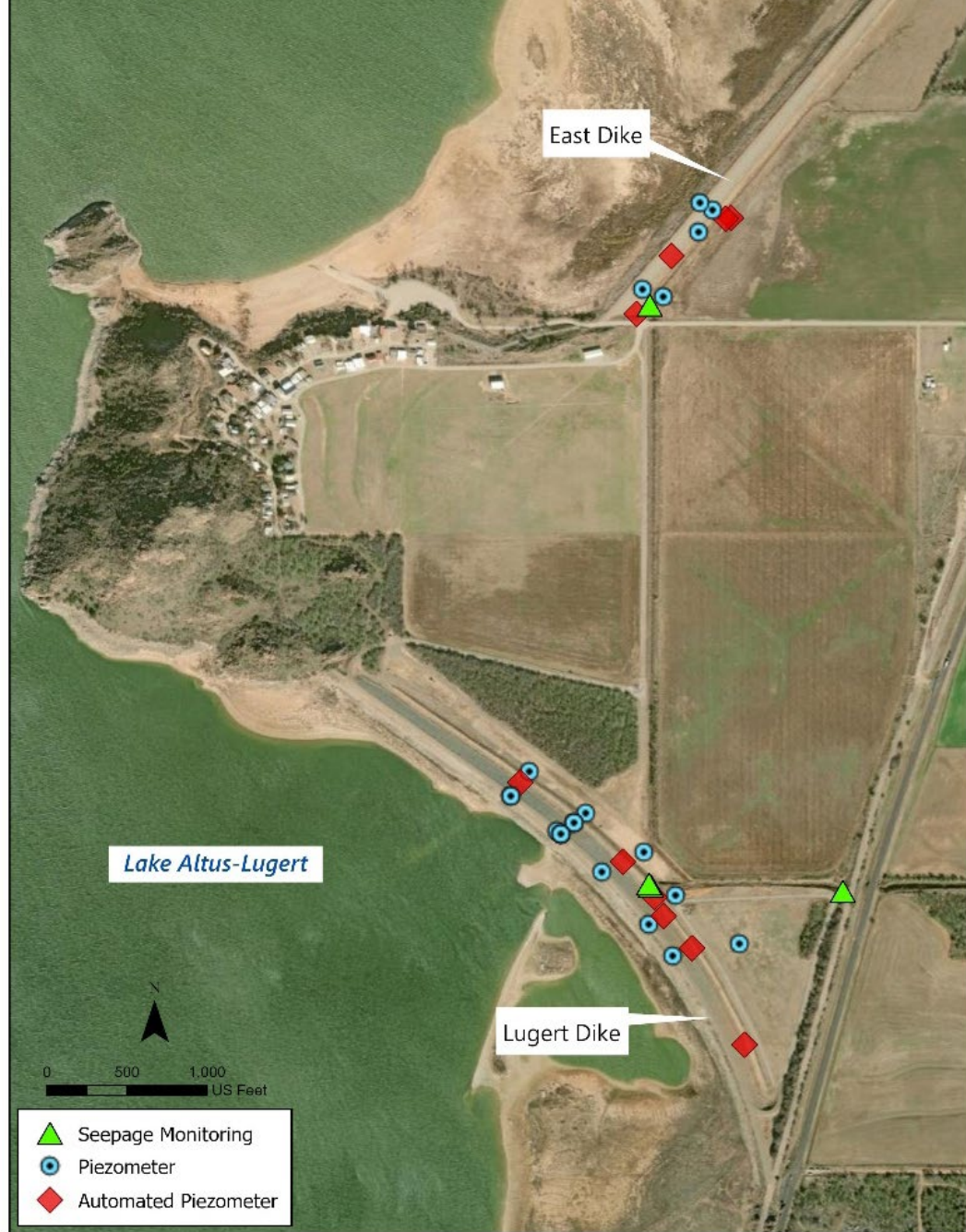
Piezometers and seepage measurement devices at Lugert and East Dikes.
