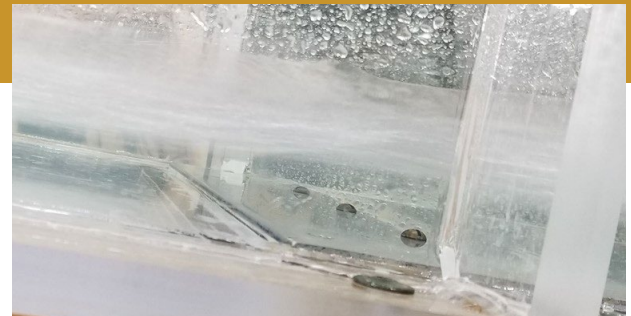
Flow over spillway offsets: (top) attached to floor at a small offset and (bottom) detached from floor at a large offset.
