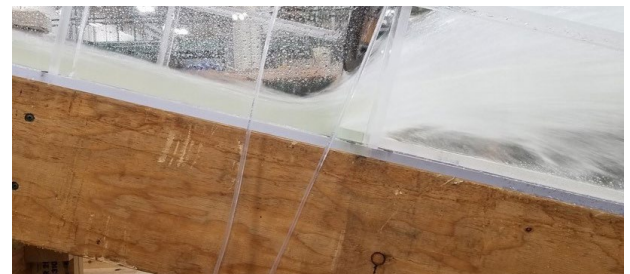
Flow over spillway offsets: (top) attached to floor at a small offset and (bottom) detached from floor at a large offset.
