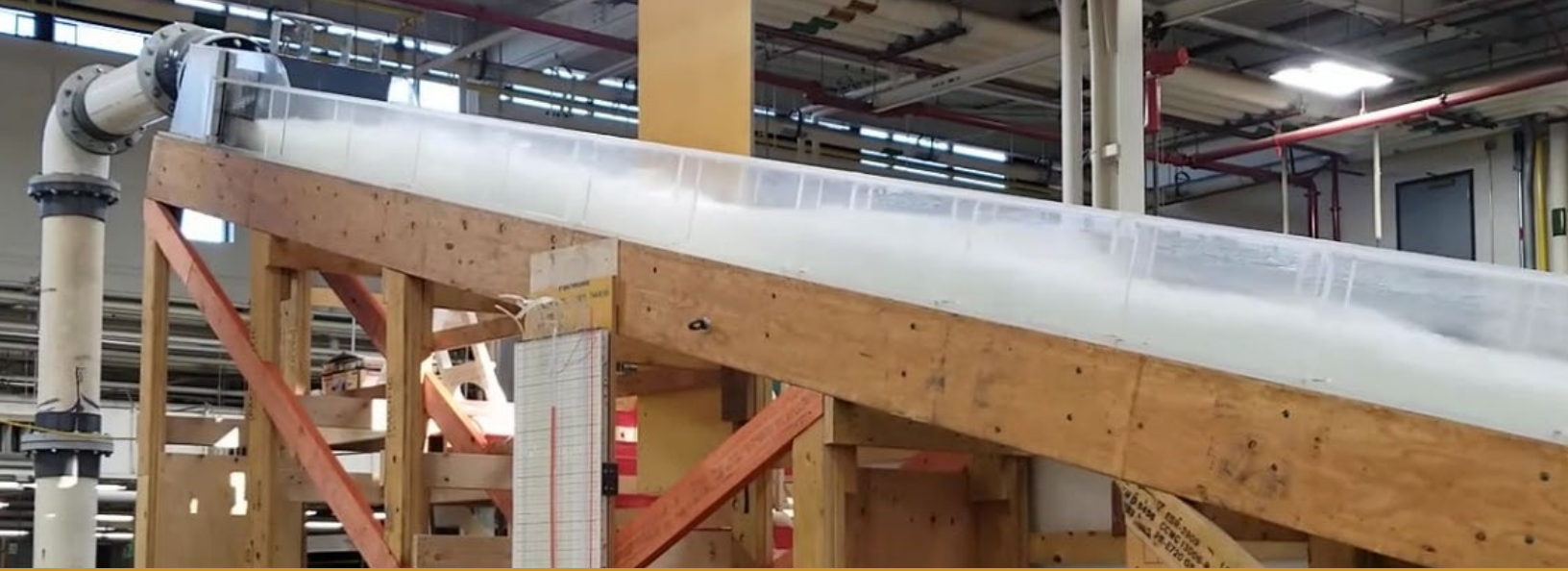
Hydraulic jacking research flume constructed and operated as part of the Technology Development Program.
