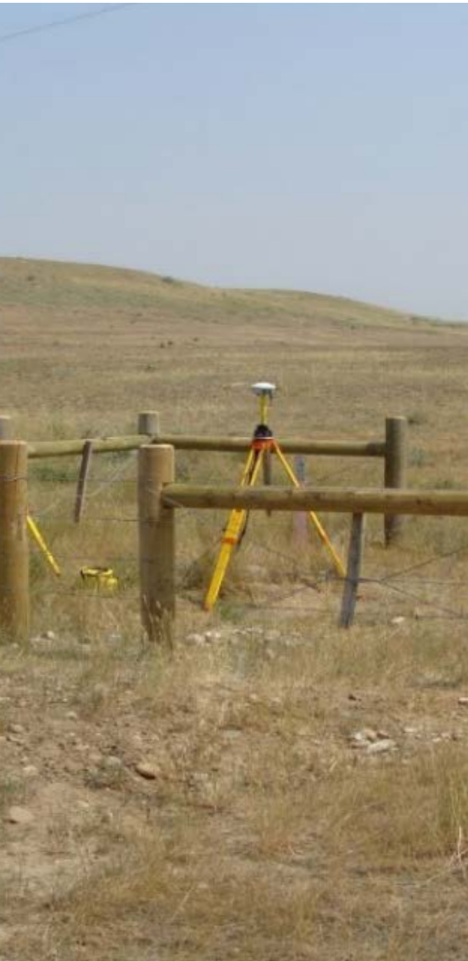
Protective fencing for survey control point NDA-1 (1993) at Nelson Dikes, Montana.
